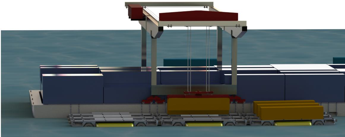
Figure 11: Visualisation of unloading of AAGVs in grid format to Floating Terminal
