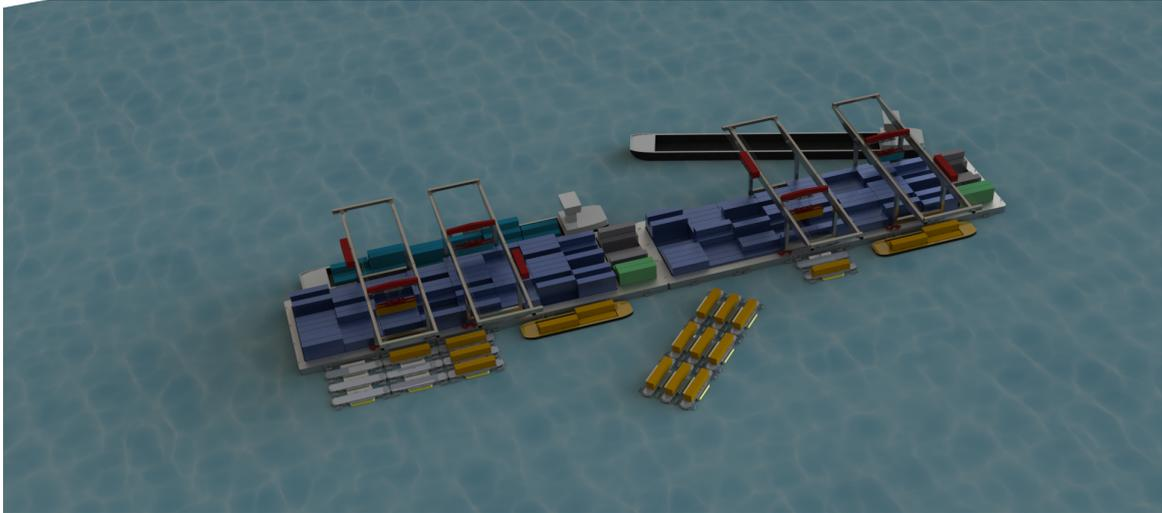
Figure 12: Visualisation of modularity of concept, 2 Floating Terminals and multiple configurations of AAGVs
