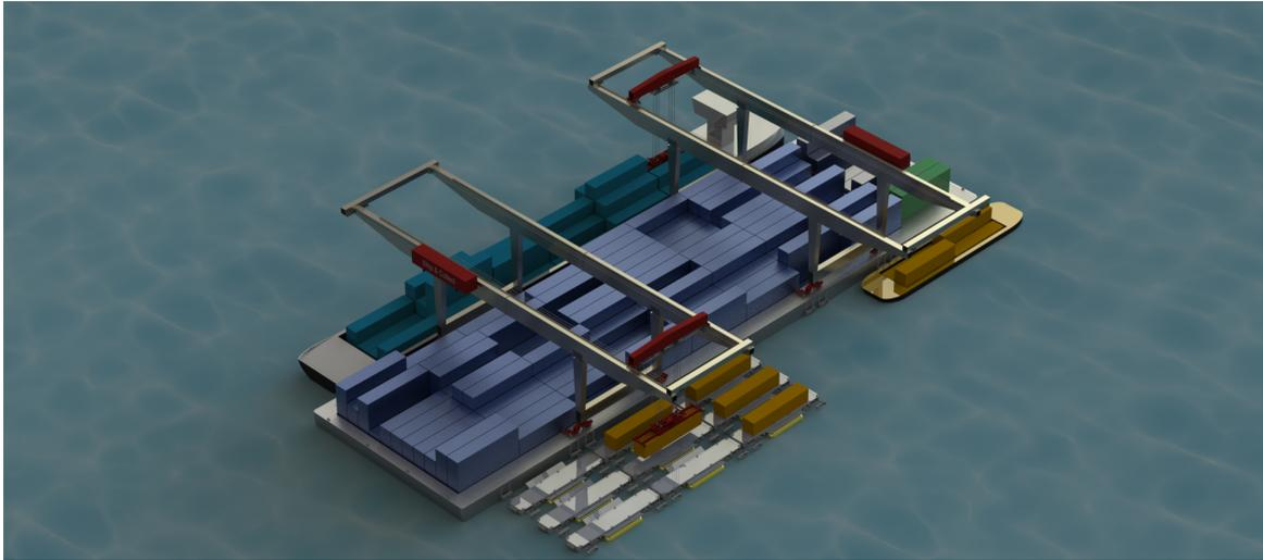
Figure 10: Overview of grid of AAGVs docked at Floating Terminal
