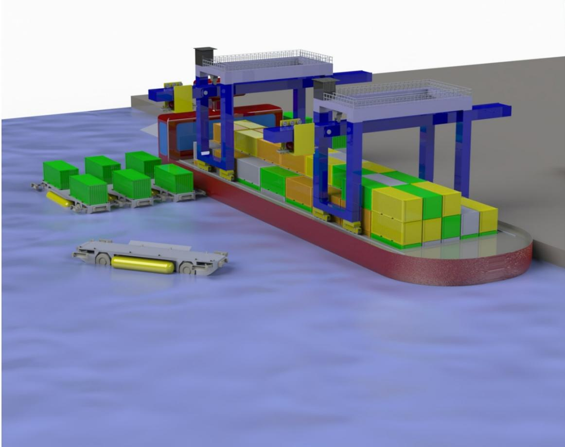
Figure 24: Visualisation of on-water container transfer AAGV to D.O.P.E.
