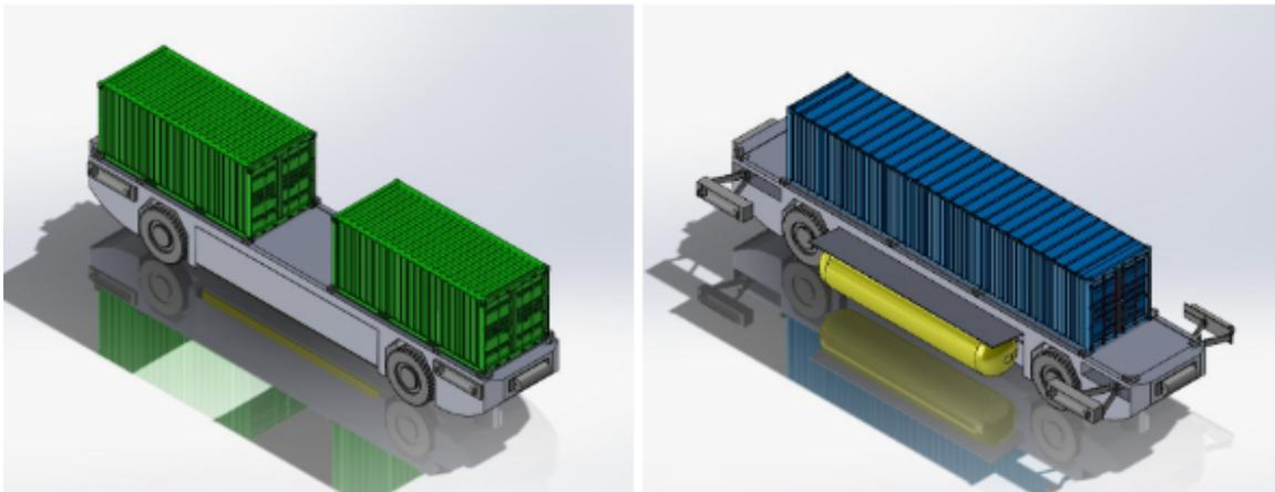
Figure 2: Final design AAGV in land mode (left) and water mode (right)
