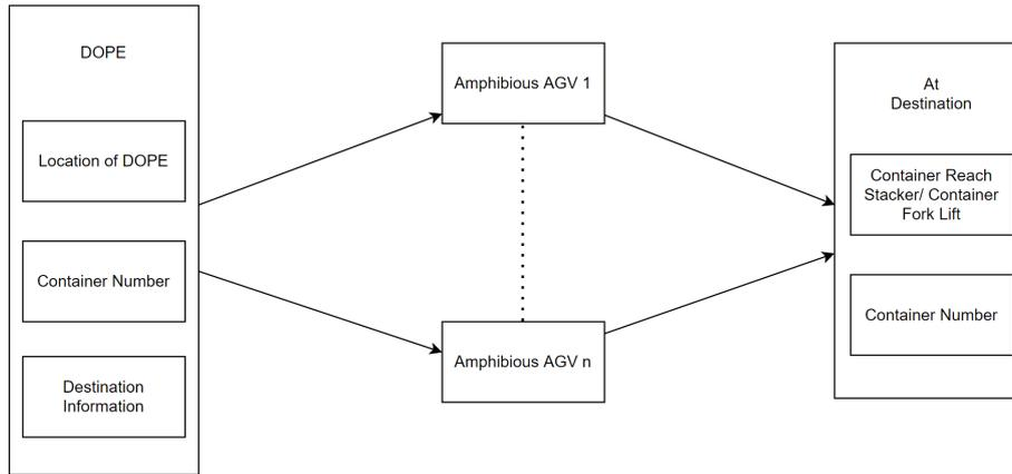
Figure 30: Control System between DOPE and Amphibious AGVs
