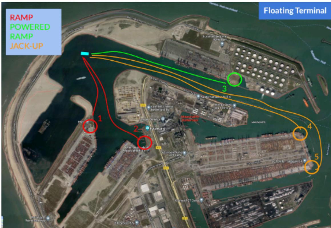
Figure 9: Floating Terminal placement and AAGV transfer points (magnification factor of 1.5)
