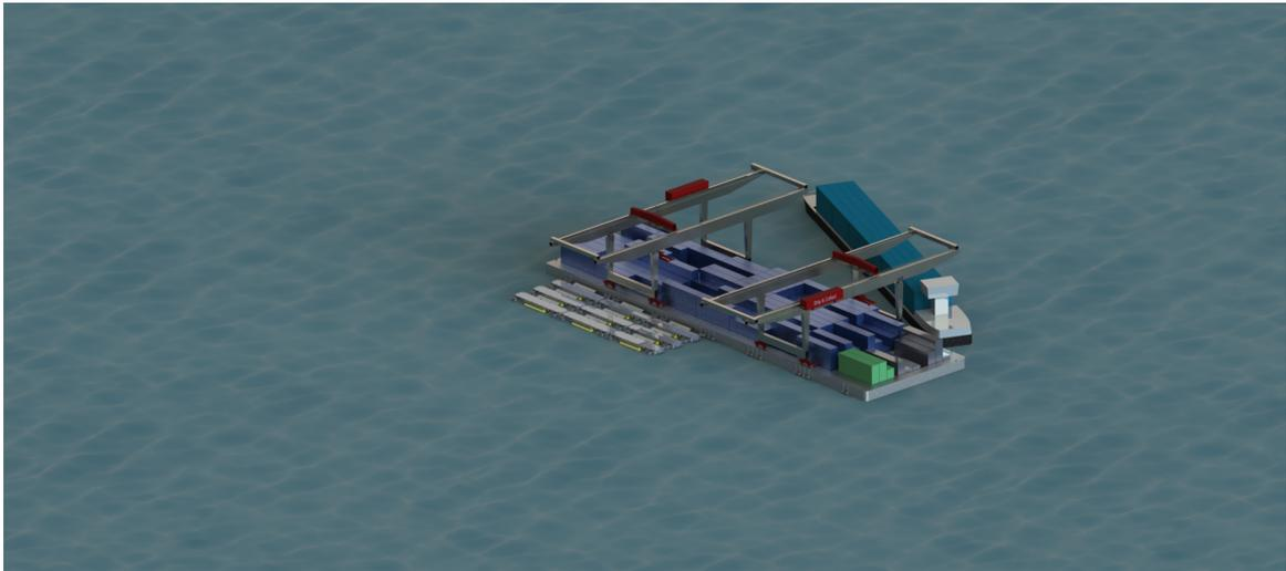
Figure 14: Departure of inland barge from Floating Terminal after unloading from 3x3 grid format AAGV
