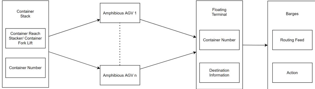
Figure 21: Control System between Floating terminal and Amphibious AGVs
