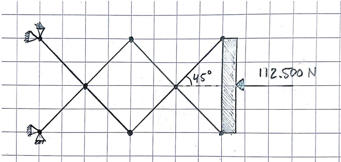
Figure 33: Schematic of force acting on AAGV scissor mechanism situation 1
