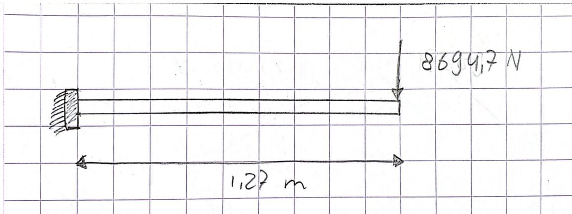
Figure 34: Schematic of simplified situation weight of electromagnet
