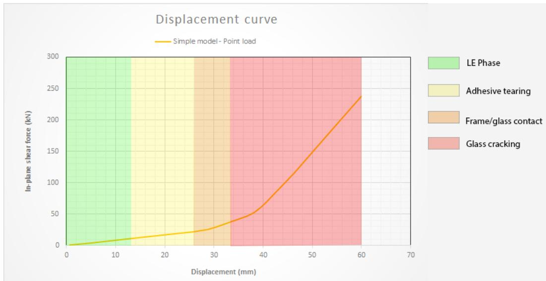
Figure 30: Displacement curve of Model 1
