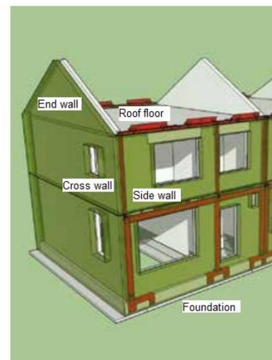
Figure 8: 3D View of a house (Roijsackers et al., 2017)
