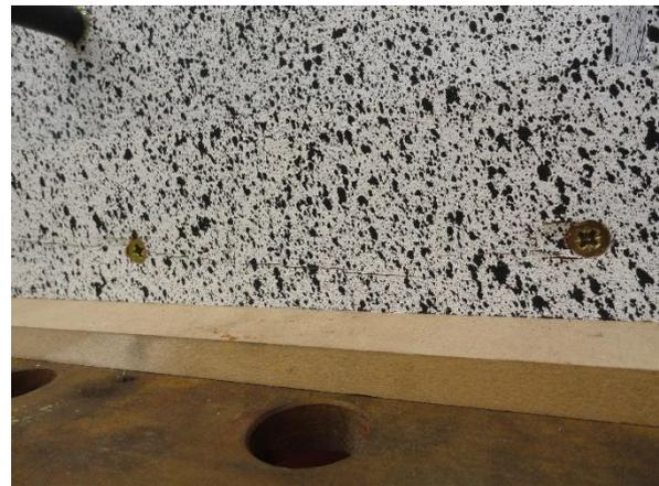
Figure 55: Left: Crack of the upper timber bar, Right: Cracking of the lower timber bar
