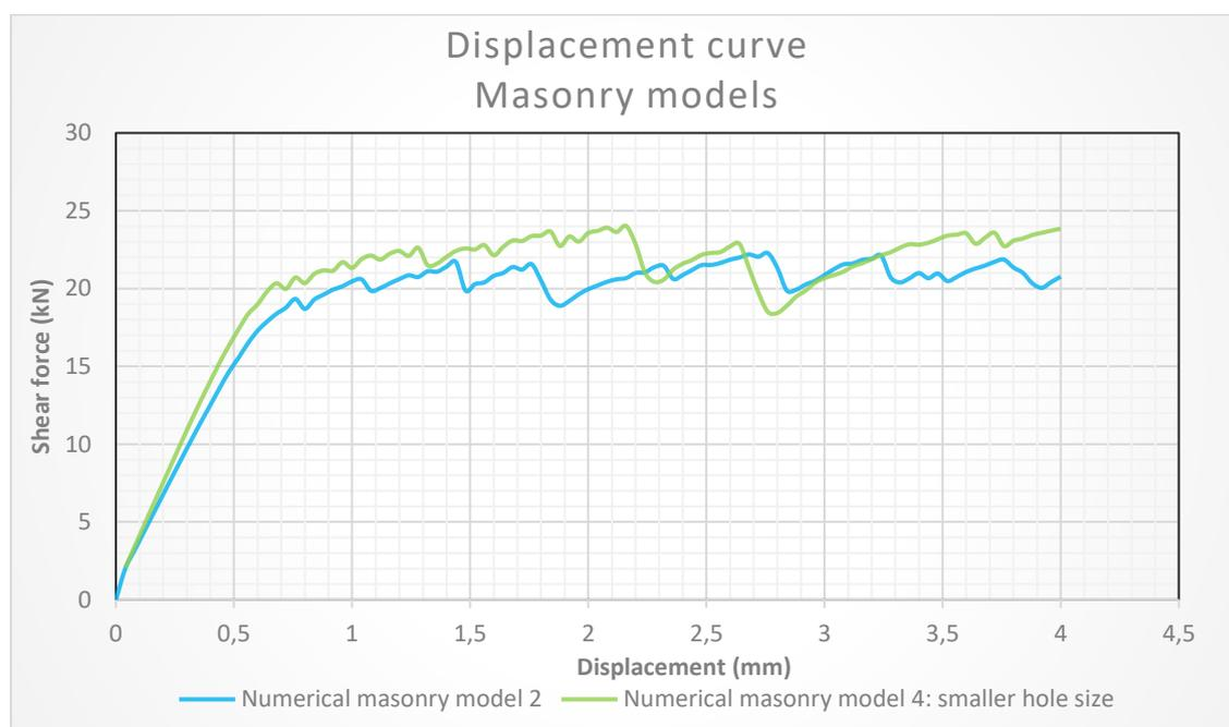
Figure 76: Displacement curve masonry walls
