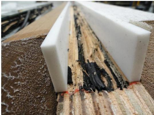
Figure 54: Pinching of the timber frame
