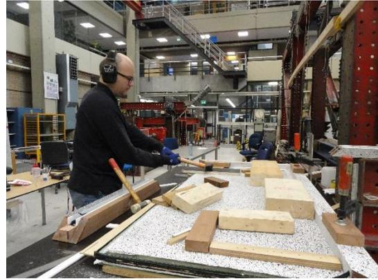
Figure 53: Left: detaching of the timber frame with a hydraulic pump, Right: detaching the timber frame with a hammer
