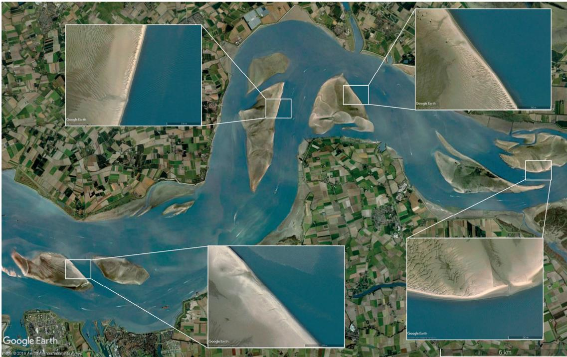
**Figure 2.2.** Google Earth satellite images showing small-scale levee formations at the channel-shoal interface in the WS. Note: Large and small images scales (bottom right) are 6 km and 200 m, respectively.
