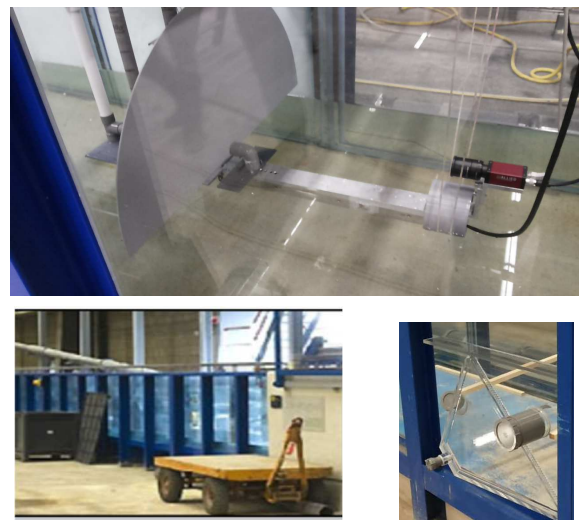
Figure 1: Rotation structure (up), the flume (down left) and a window with lateral connection (down right) along the flume.
