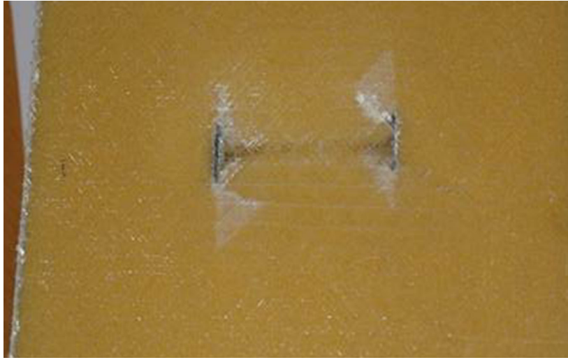
Figure 4.1: Damage after the point load test on a 25 mm glass fibre foam sandwich sample.
