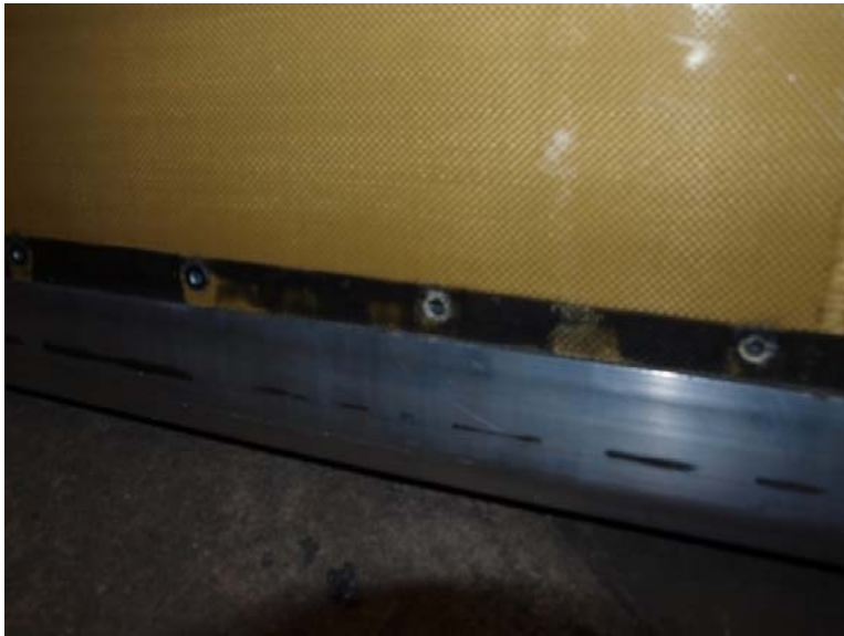
Figure 5.19: Five rivets were found to be missing after the test.
