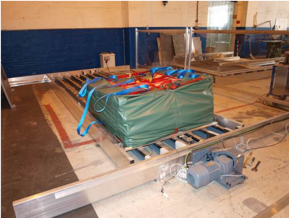
Figure 5.9: Photo of a prototype base on the dynamic testing rig to simulate damage and wear on an air cargo container bottom plate due to transportation rollers used in aircraft.
