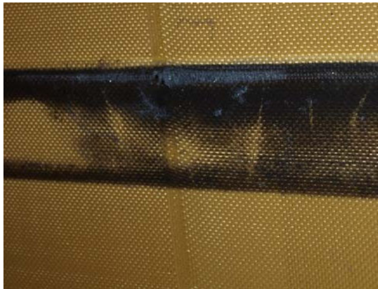
Figure 5.15: Close-up of the wear due to the rollers and structure on the aramid plate.
