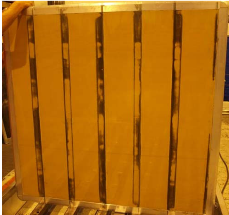
Figure 5.14: Visible wear lines where the rollers and structure made contact with the aramid plate.
