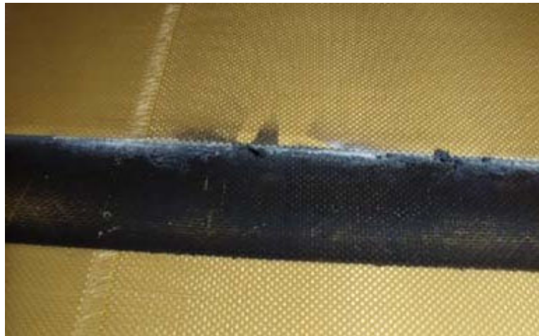
Figure 5.18: Close-up of the wear due to the rollers on the felt plate.
