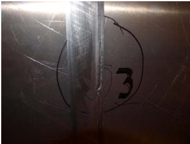
Figure 5.12: Visible crack in the aluminium plate after testing.
