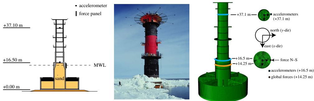
Figure 2. Illustration, picture and finite-element model of the Norströmsgrund lighthouse (from Nord et al. [26]). (Online version in colour.)
