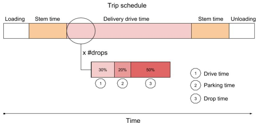
**Figure 4-4:** Schematic breakdown of a trip: the white parts indicate the (un)loading time of the frames, orange parts are the stem time to and from the delivery area, and the red part is the delivery drive time. The delivery drive time consists of a repetitive sequence for every customer with: drive time, parking time and drop time.
