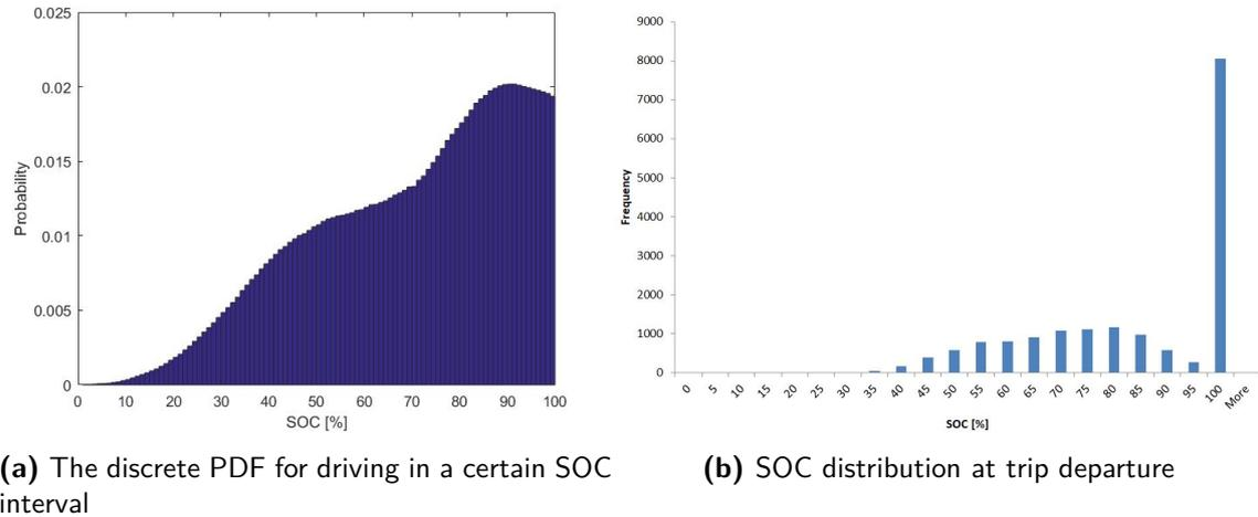
**Figure 4-6:** SOC cycling ranges and SOC at trip departure
