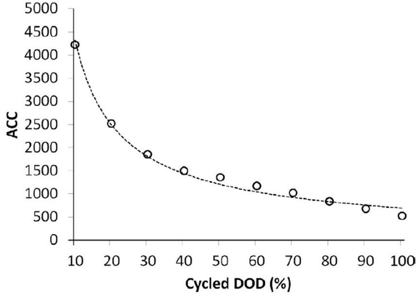
**Figure 2-1:** ACC-DOD curve. Each marker represents a sample point where the achievable cycle life is known. The continuous line shows the best fit curve of the ACC data. [38]
