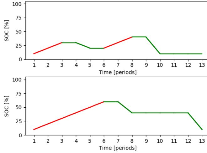
**Figure 3-3:** Visualised vehicle SOC for experiment 1: red lines indicate the periods in which the vehicle is being charged.
