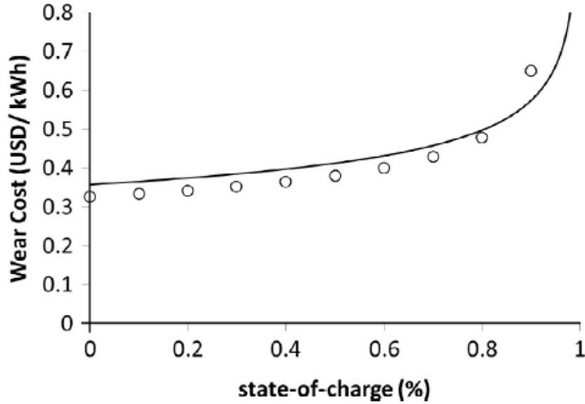
**Figure 2-2:** Discrete and continuous wear costs functions derived by using the ACC-DOD data from Figure 2-1
