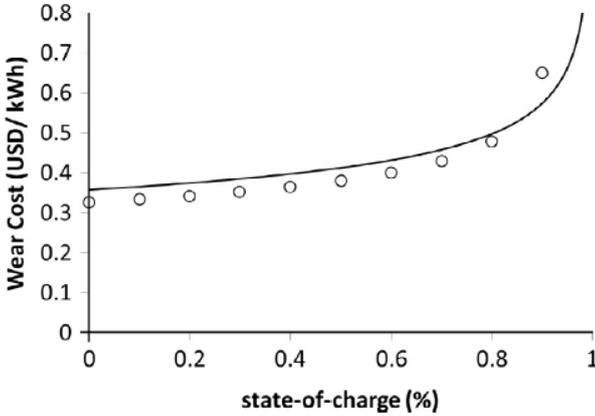
Fig. 2: Discrete and continuous wear costs functions derived by using the ACC-DOD data from Figure 1 [12]
