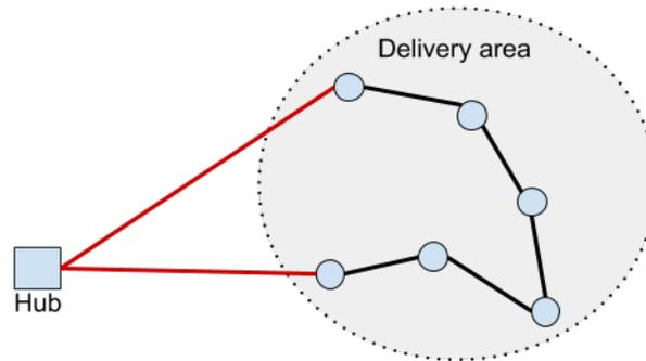
**Figure 4-3:** Overview of a trip: the red lines indicate the drive time to the delivery area, also known as stem time. When arrived in the delivery area, a set of customers is served after which the vehicle returns to the hub
