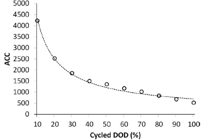
Fig. 1: ACC-DOD curve. Each marker represents a sample point where the achievable cycle life is known. The continuous line shows the best fit curve of the ACC data. [13]
