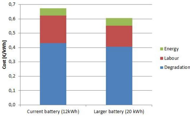
Fig. 8: The impact of an increased battery size
