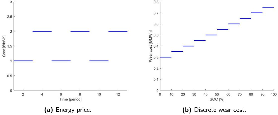
**Figure 3-2:** Energy cost and wear cost function.
