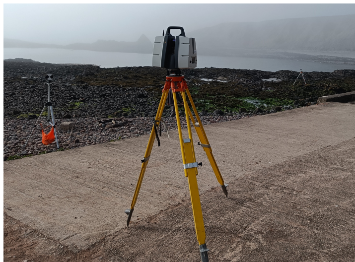
Figure 2.4: Example of a ToF laser scanner, the Leica ScanStation P40, on a tripod.
