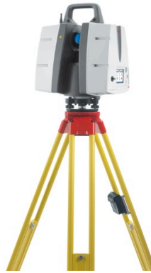
Figure 5.5: The Leica P40 Laser Scanner on top of a tripod. This specific model is used during the field work acquiring the point clouds. Image from CR Kennedy.
