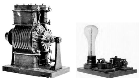
Figure 73: Maxim's dynamo (left) and incandescent, graphite, lamp (1878)/
