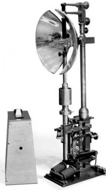
Figure 39: Serrin regulator for a carbon arc light (1857).
