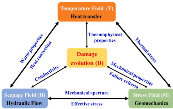
Fig. 1. Thermo-hydro-mechanical and damage (THM-D) coupling mechanism.
