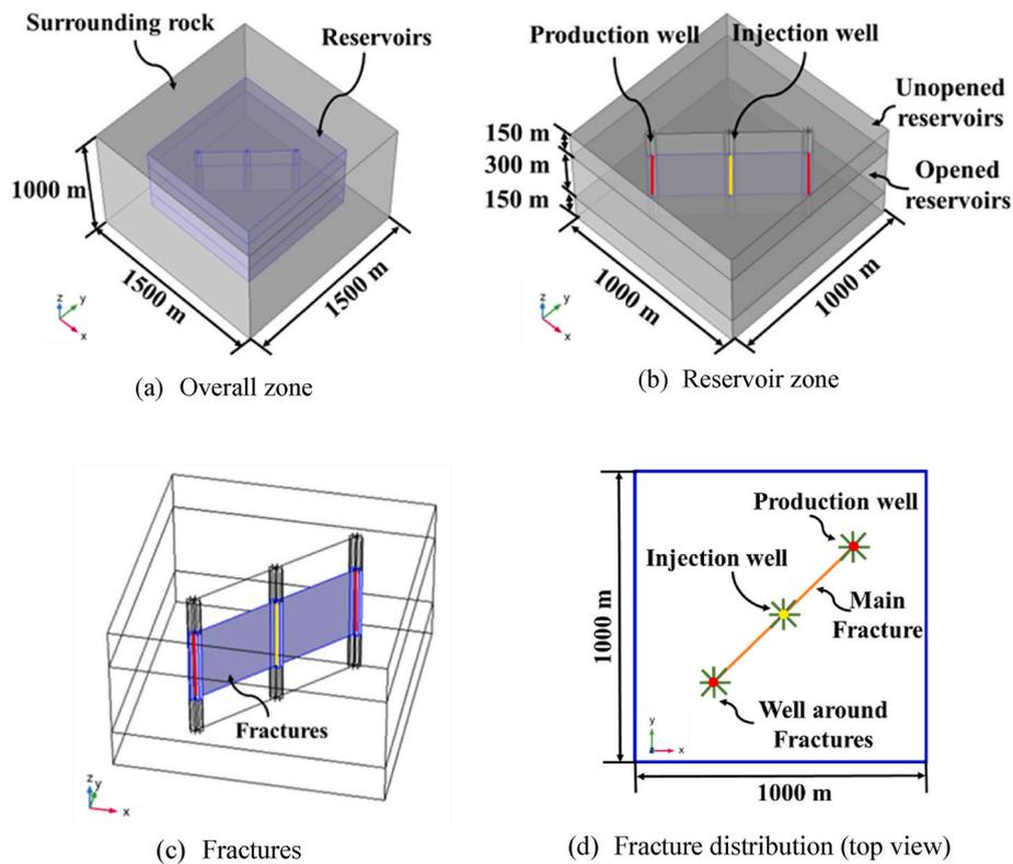
Fig. 4. Computational zone for the numerical model.
