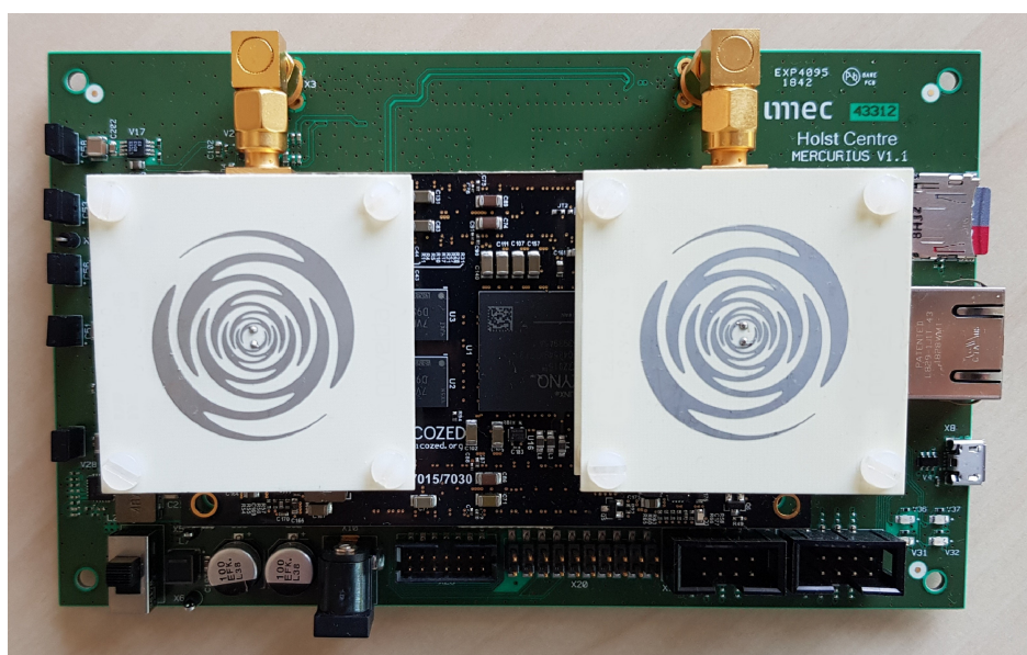
Figure 7.1: Radar-based sensor to be used in the acquisition of the Doppler signals
