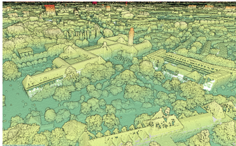
(a) AHN4 LiDAR point cloud
