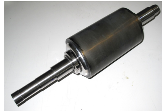
Figure 2-10: Rotor structure with Halbach array.
