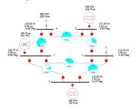
Fig. 1. Load flow simulation results: PowerWorld.
