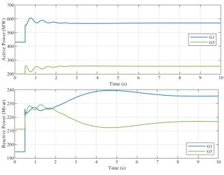
Fig. 10. Real-time time-domain simulation, ePHASORSIM: Generated active (top) and reactive (bottom) power of G1 and G5.
