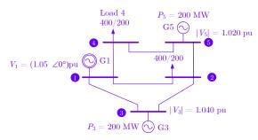
Fig. 1. Single line diagram of -bus test system -Mesh: Test System.
