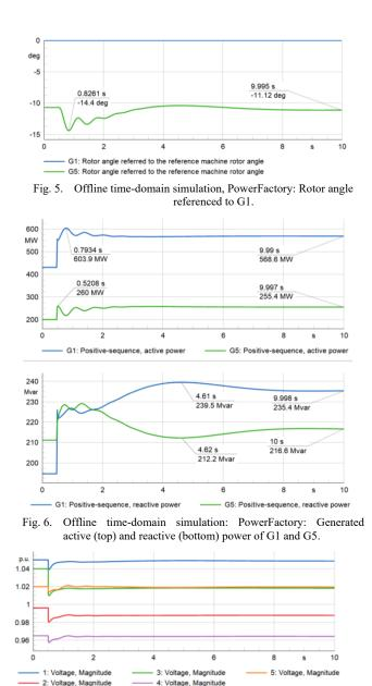
Fig. 7. Offline time-domain simulation: PowerFactory: Voltages at the busbars (per unit).
