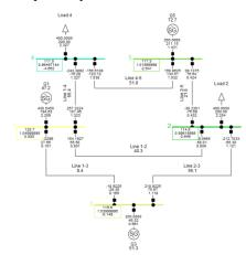
Fig. 2. Load flow simulation results: DIgSILENT PowerFactory
