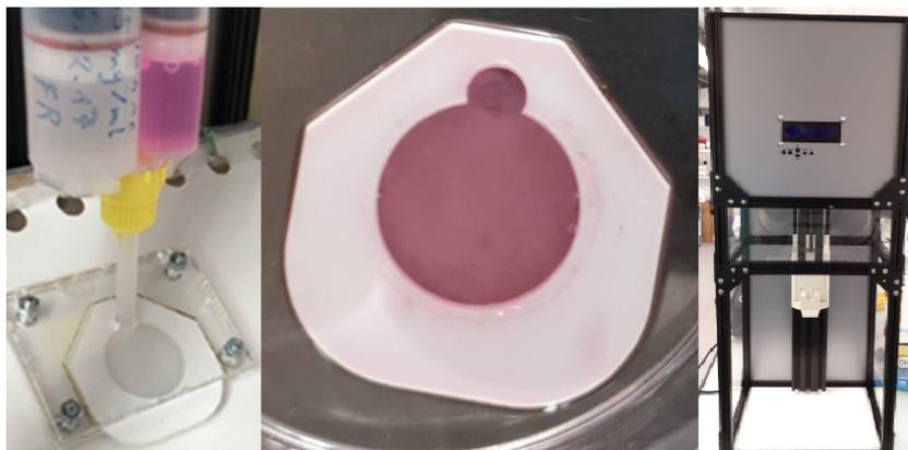
Figure 1.7: Components of injection molding process. Left: Double cartridge, containing high concentration collagen in the left container and fibroblasts suspension in the right container, along with a mixing nozzle in which the contents are mixed and then injected into the encased mold. Middle: in-mold dermal hydrogel (pink colour due to fibroblasts culture medium). Right: Device for automated fabrication of dermal equivalents.
