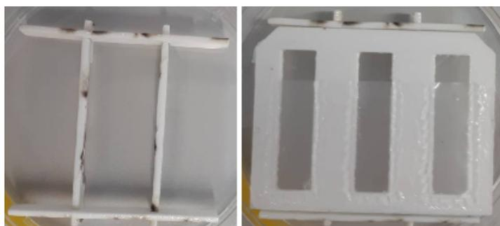
Figure 2.2: Assembled polystyrene holders used to lift the molds at the air-liquid interface. Assembled holders without the mold (left) and with the mold (right).
