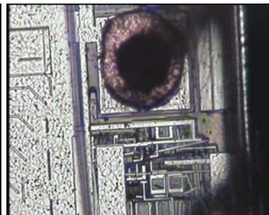
Figure 13. Damaged patterns on the die
