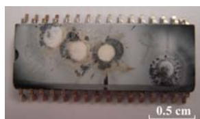
Figure 3. Profile after Ar+O 2 plasma etching
