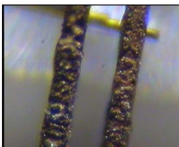
Figure 11. Intentionally damaged Cu wires
