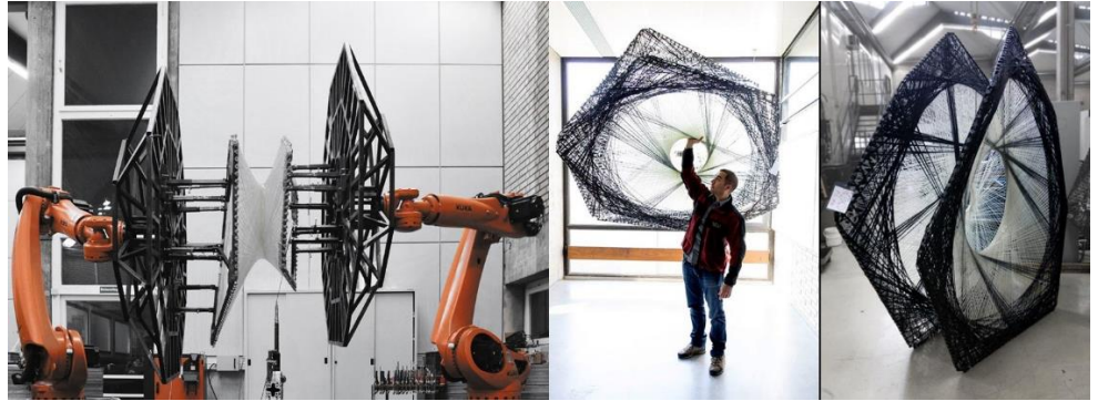
Figure 10. manufacturing of the Elytra pavilion modules (source: icd.uni-stuttgart.de).
