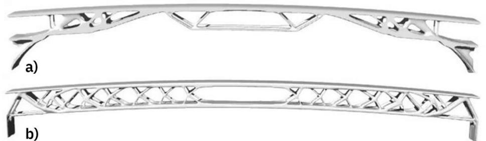
Figure 39. influence of support conditions on TO results by BESO a) both supports pinned; b) one pin and one roller support. (source: Xie et al., 2011)
