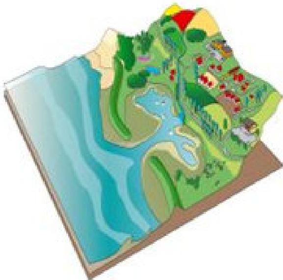
Figure 3-8: Example from the Comcoast project of a coastal development zone that combines flood protection and nature development.
