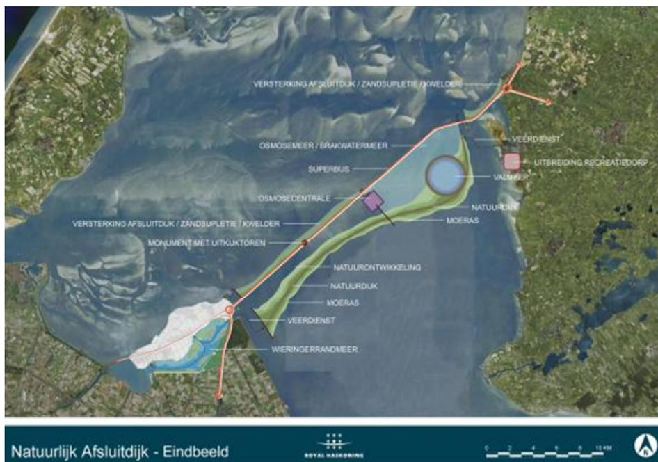
**Figure 3-6: One of the proposed designs for the Afsluitdijk / closure dam in the Netherlands, with several additional functions, such as nature development and tidal energy generation.**
