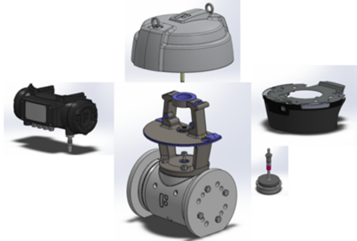
Figure 3.2: Left: E-house, Top mid: Actuator, bottom mid: Body, top right: Cover and bottom right: Plug and seat. Source: FOCUS-ON
