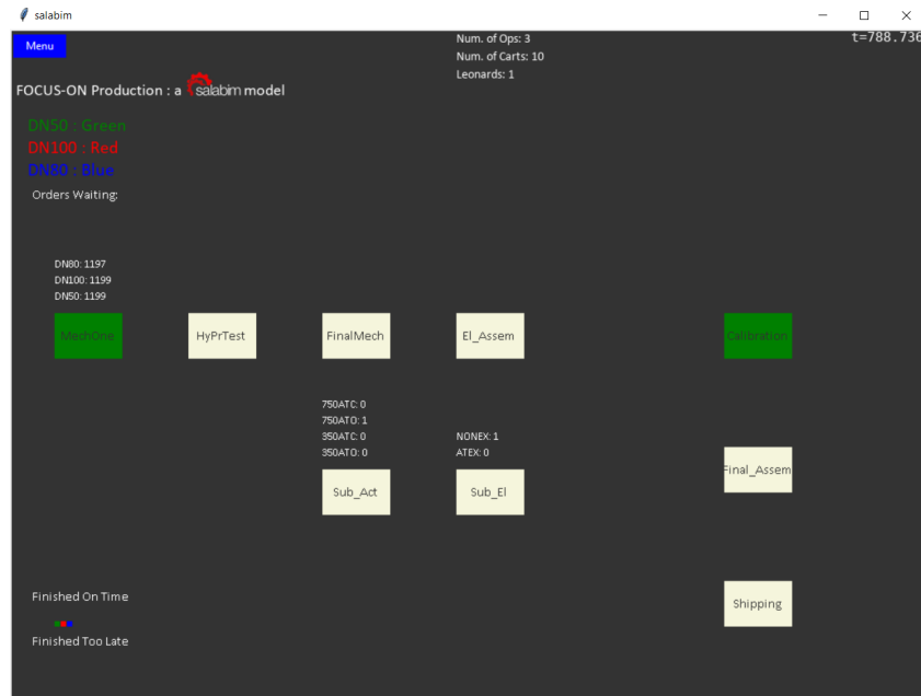
Figure 5.2: Animation window of the DT model of the FOCUS-1 Production line: a schematic view.
