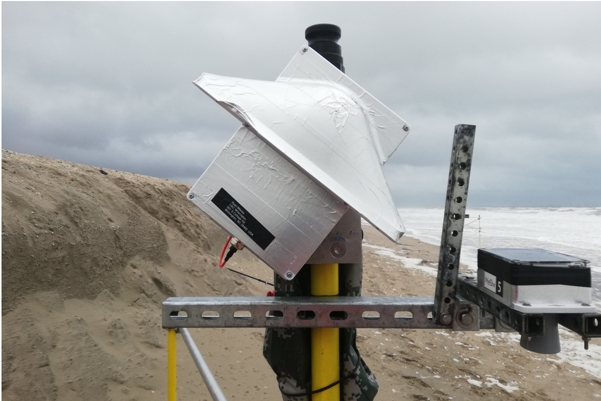
Figure 2.24: Image of the LLC LiDAR during the Fieldwork Experiment. The LLC LiDAR is inside the silver box with the triangle shaped extension. This is a water tight cover to protect the instrument from wave impact. The other instrument, located on the bottom right of the image, has not been used in this MSc Thesis.
