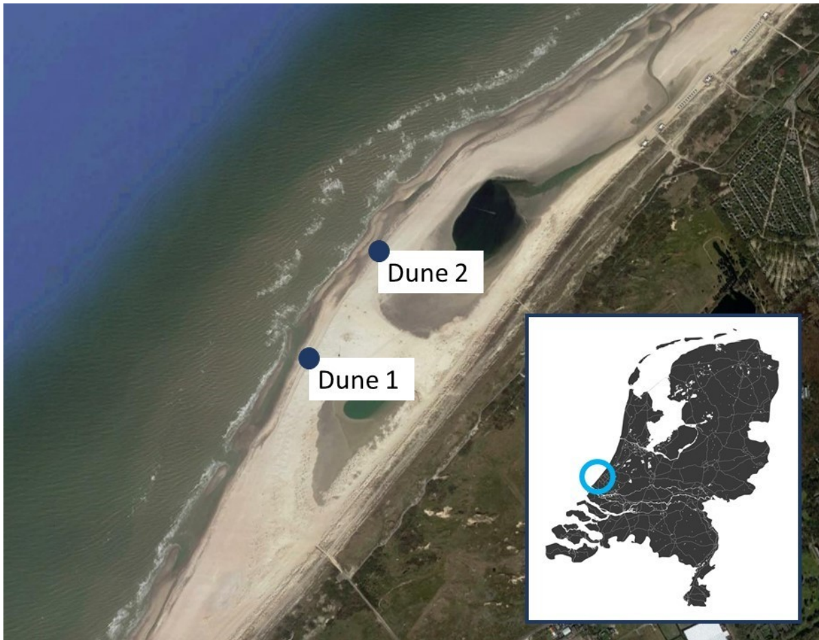
Figure 2.2: The image gives an overview of the sand engine and artificial dunes created for the experiment. The small chart on the bottom right indicates the location of the Sand engine within the Netherlands.
