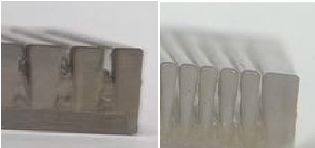
Figure 2: two typical air channels collapsed. Top of the channel is open and Substrate material flows down in the channel.
