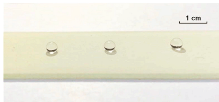
Figure 7. Hydrophobic performances of the super-hydrophobic coating after the sandpaper wearing test.
