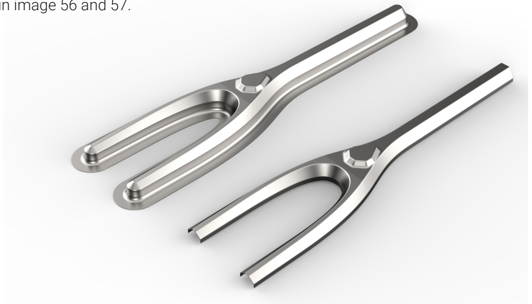
Image 57: Simulated and trimmed part
