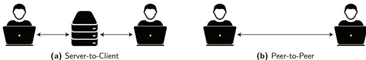
Figure 2-1: Difference between Server to Client and Peer to Peer communication
