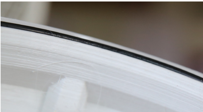
J.3. Visible moisture on O-ring
