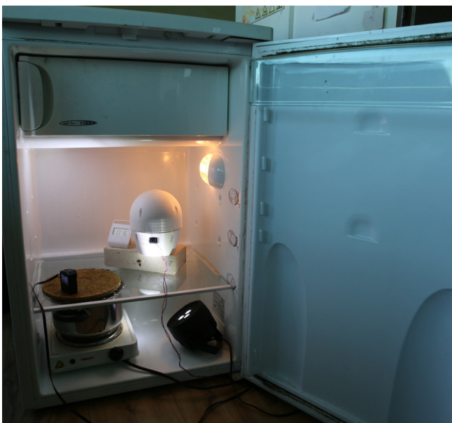
1.2. ↖ Repaired 3D printer has been printing continuously for 30 - ↗ Rain testing in the shower ↙ Refrigerator as climate chamber - ↘ Testing a solar system out of the living room window.
