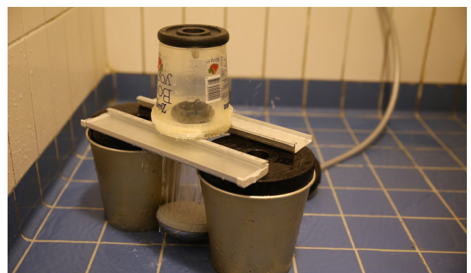
I.4. Drain element sprayed with showerhead
