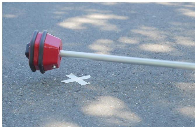
6.45. ROVER2 model seemingly undamaged after fall on asphalt.
