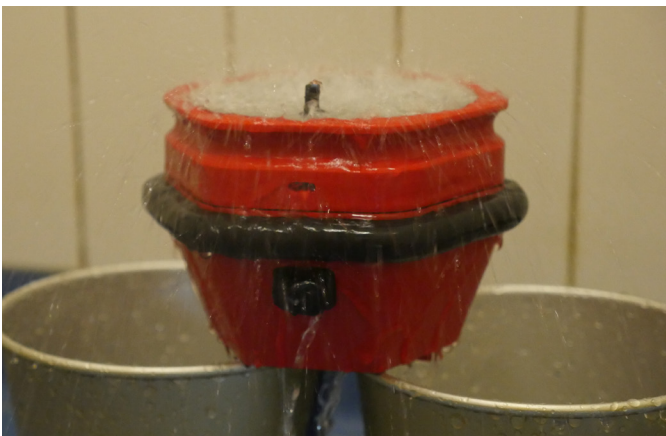
6.23. ROVER2 in the 15-minute rain test using the shower.
