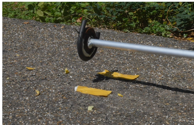
6.47. Testing the dampening effect of several rubber profiles with high speed footage.
