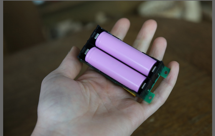
6.41. Rover battery lithium-ion cells.
