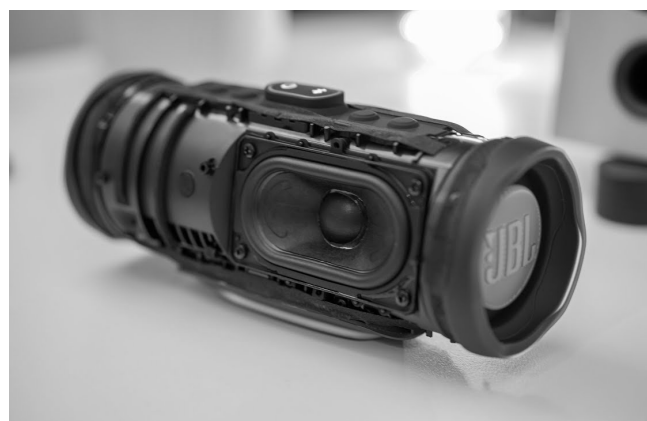
6.18. Connection between speaker and housing is closed off using a gasket.
