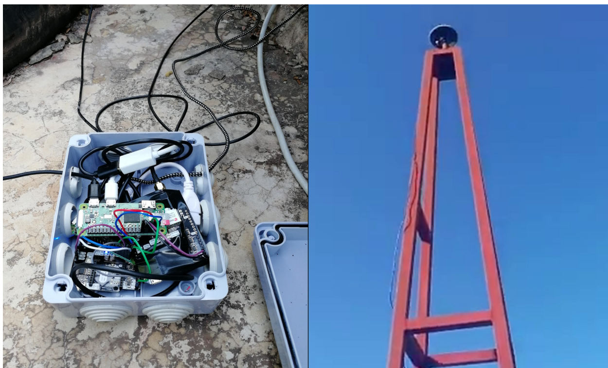
image / figure 2: Current state of the base station; left: the electronics, right: its fixed location antenna
