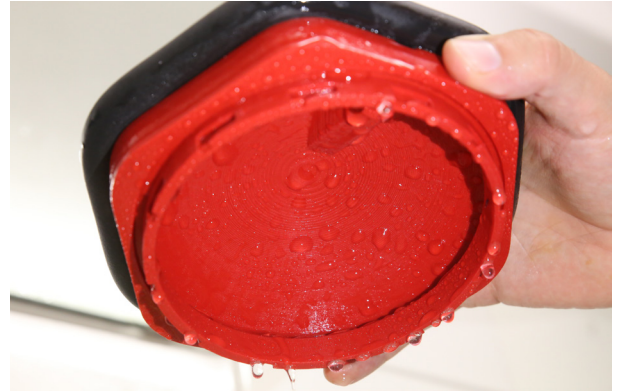
6.16. Drops of water roll down following the curved roof surface of the ROVER2 housing.
