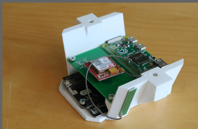
6.30. Sim800L and antenna on BASE1 electronics rack.
