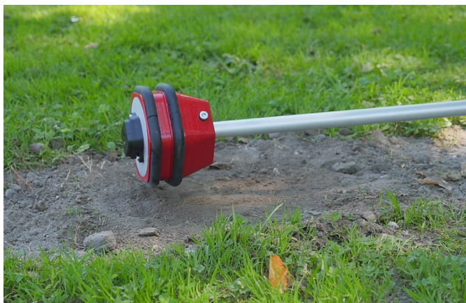
6.44. ROVER2 model undamaged after fall on sand
