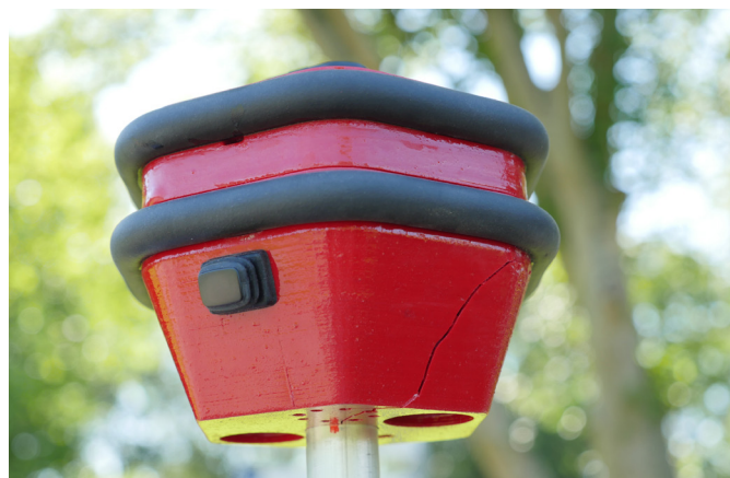
6.46. ROVER2 lower rover housing cracked after fall on asphalt.
