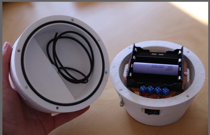
6.20. ROVER1, O-ring in a groove which can be tightened with 4 bolts
