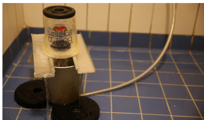
I.3. Drain element sprayed directly with tap water
