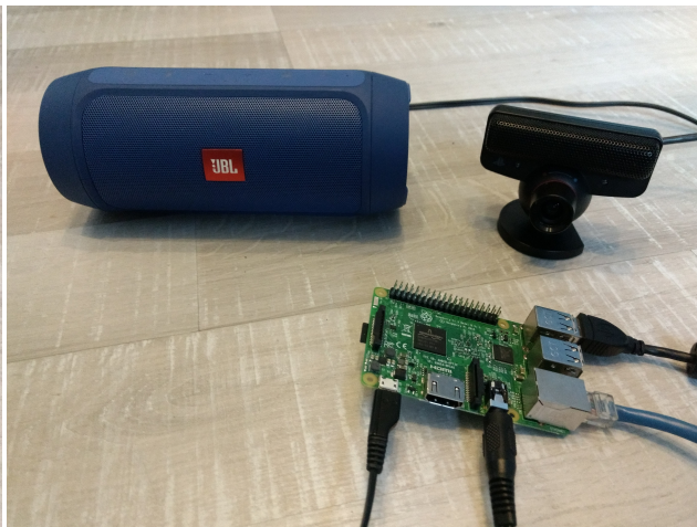
(b) Benchmark setup of Mycroft running on a raspberry pi (Picroft), external microphone, and speakers
