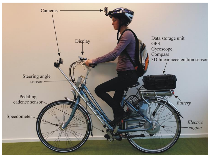
Fig. 5.1. The instrumentation of the pedelec. The instrumented conventional bicycle was not fitted with the battery and electric engine (indicated in italics).
