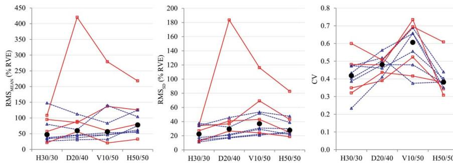
**FIGURE 6** EMG variables for the dominant upper trapezius muscle in the four workstation designs at the MAWP:  $RMS_{MEAN}$  (left),  $RMS_{SD}$  (middle), and CV (right). Lines show individual results for females ( $n = 4$ , red squares, solid lines) and males ( $n = 6$ , blue triangles, dashed lines); median values across all participants are marked by black circles.
