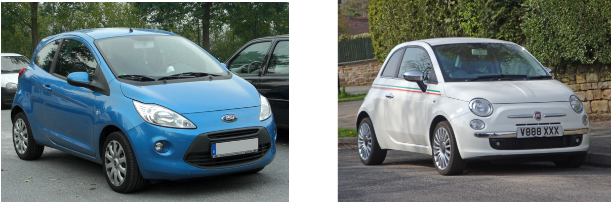
Figure 3.1: Ford Ka (left) and Fiat 500 (right) sharing the same underbody
