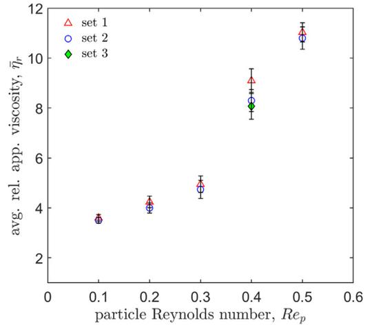
**Fig. 7.** Average relative apparent viscosities (computed from top and bottom wall) of the suspensions at varying shear rates (and therefore  $Re_p$ ) at a constant confinement ratio  $\delta = 0.17$  for several random initial configurations of the particles. The third set (filled symbol) was computed only for  $Re_p = 0.44$ . For all cases,  $\phi_v = 38\%$  and the errorbars show the standard deviations of the fluctuations.
