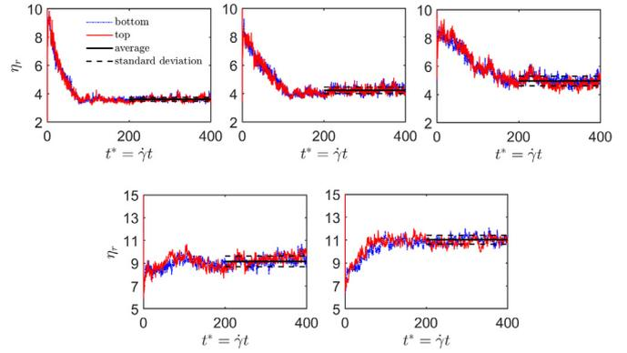
**Fig. 6.** Relative apparent viscosity of a rigid sphere suspension as a function of time obtained for one random initial particle configuration (set 1) with  $\phi_v = 38\%$ . Top row:  $Re_p = 0.11, 0.22, 0.33$ . Bottom row:  $Re_p = 0.44, 0.55$ . (For interpretation of the references to colour in the text, the reader is referred to the web version of this article.)
