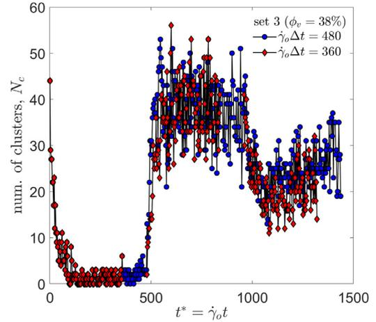
**Fig. 14.** Evolution of particle clusters over time for a suspension with 38% solids. The particle Reynolds number switches between 0.33 in zone 1 to 0.55 in zone 2, and back to 0.33 in zone 3. The suspension is sheared for a time interval  $\dot{\gamma}_0 \Delta t = 360$  in each zone of the shorter simulation and  $\dot{\gamma}_0 \Delta t = 480$  in the longer simulation. (For interpretation of the references to colour in text, the reader is referred to the web version of this article.)
