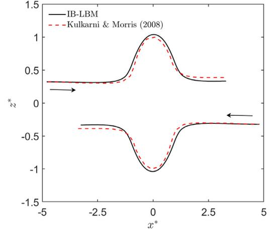
**Fig. 4.** Trajectories of two particles in simple shear flow at  $Re_p = 0.1$ . Solid and dashed lines show the simulation results obtained by the present IB-LBM code and [Kulkarni and Morris \(2008\)](#), respectively.  $x^*$  and  $z^*$  are the particle positions scaled by particle radius and relative to the centre of the domain. Arrows indicate the direction of the motion.
