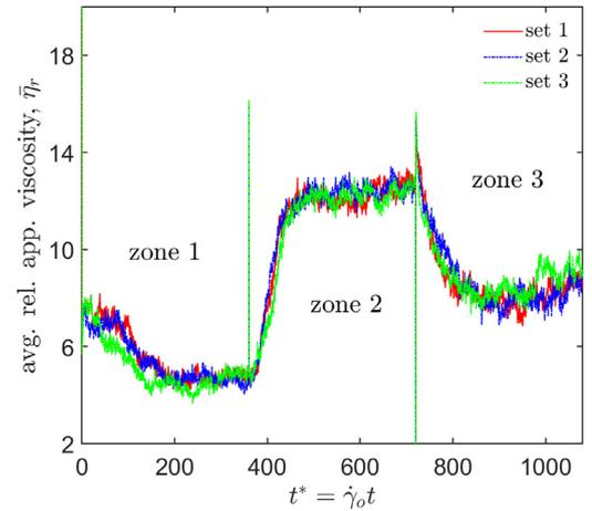
**Fig. 12.** Fluctuations in the average relative apparent viscosity of the suspension as a function of time in a simulation with a varying shear rate computed for three random initial states. The particle Reynolds number changed between 0.33 in zone 1, 0.55 in zone 2, and back to 0.33 in zone 3 with  $\phi_v = 38\%$
