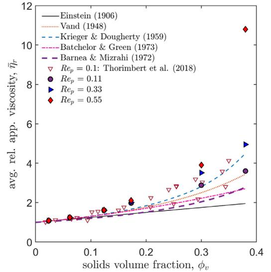
**Fig. 9.** Average relative apparent viscosities of suspensions with varying solids volume fractions (computed based on  $R_{hyd}$ ) as determined by theoretical and empirical expressions (solid and broken lines) and IB-LBM simulations (present work: filled symbols). The simulations of Thorimbert et al. (2018) at  $Re_p = 0.1$  are also included (open triangles).
