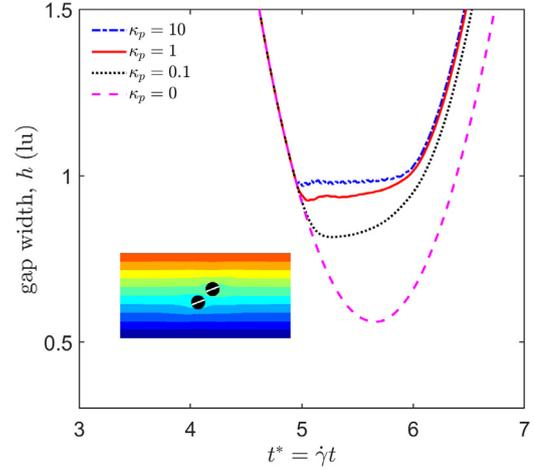
**Fig. 2.** Gap width between two colliding particles as a function of time for several repulsive force strengths  $\kappa_p$ . Inset: sample visualisation of the cross-section through the colliding particles at an instant of time after the collision. The background is coloured according to the  $x$  component of the liquid velocity. (For interpretation of the references to colour in this figure, the reader is referred to the web version of this article.)
