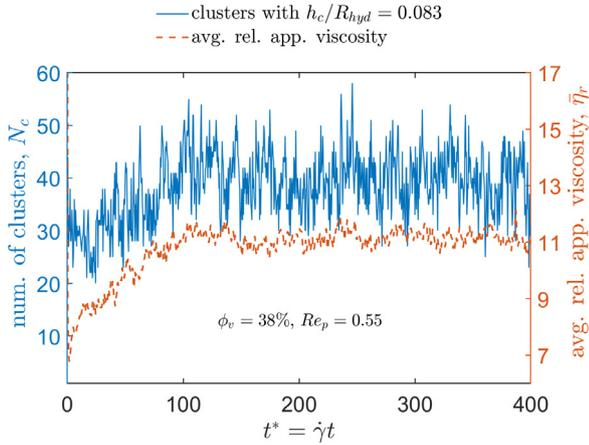
**Fig. 11.** Evolution of the number of clusters and the relative apparent viscosity (average of top and bottom wall) as a function of time. The cluster threshold is  $h_c/R_{hyd} = 0.083$ ,  $Re_p = 0.55$ , and  $\phi_v = 38\%$ .
