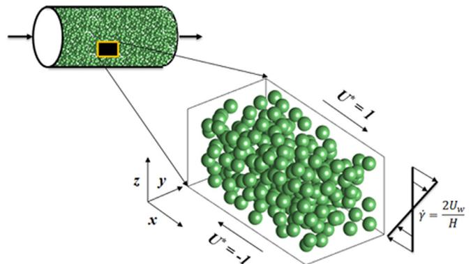
Fig. 1. Schematic of the simulated monodisperse suspension.  $U^* = U_x/U_w$  is the dimensionless fluid velocity with  $U_x$  being the  $x$  component of the fluid velocity.
