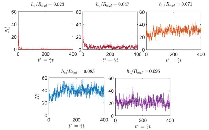
**Fig. 16.** Transient evolution of particle clusters as a function of time for several cluster cut-off distances  $h_c/R_{hyd}$  ranging between 0.02 and 0.1.  $\phi_v = 38\%$  and  $Re_p = 0.55$ .
