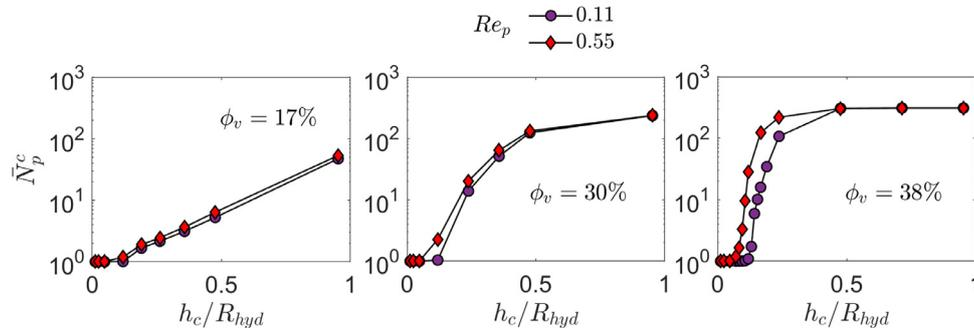
**Fig. 15.** Average cluster size as a function of cluster threshold  $h_c/R_{hyd}$  for several solids volume fractions (left to right)  $\phi_v = 17\%$ ,  $30\%$ , and  $38\%$  at  $Re_p = 0.11$  and  $0.55$ .
