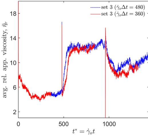
**Fig. 13.** Effect of increasing the shear time on the relative apparent viscosity of the suspension for a random initial configuration (set 3) at  $\phi_v = 38\%$ . The particle Reynolds number in these simulations switches between 0.33 and 0.55 and the duration of shear in each zone is  $\dot{\gamma}_0 \Delta t = 480$  and 360. (For interpretation of the references to colour in text, the reader is referred to the web version of this article.)
