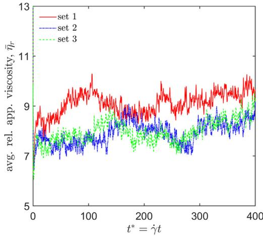
**Fig. 8.** Fluctuations in the average relative apparent viscosities of the suspension for three random initial configurations at  $Re_p = 0.44$  and  $\phi_v = 38\%$ .
