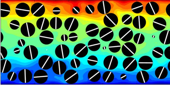
**Fig. 5.** Visualisation of a cross-section through a simulated suspension in simple shear flow ( $\phi_v = 38\%$ , and  $Re_p = 0.55$ ) at  $t^* = 17.6$ . The white lines in each circle show the orientation of the particle and the colours represent the  $x$  component of the interstitial liquid velocity scaled by the wall speed. (For interpretation of the references to colour in this figure, the reader is referred to the web version of this article.)
