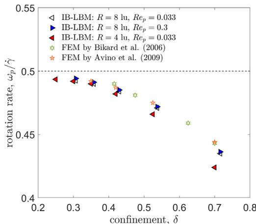
**Fig. 3.** Steady rotation rate of a particle in shear between parallel plates as a function of the confinement  $\delta$  at two different resolutions with  $R = 4$  (filled red triangles) and 8 lu (open and filled blue triangles), and  $Re_p = 0.033$  and 0.3. Dashed line shows the steady rotation rate in an unbounded domain. (For interpretation of the references to colour in this figure legend, the reader is referred to the web version of this article.)
