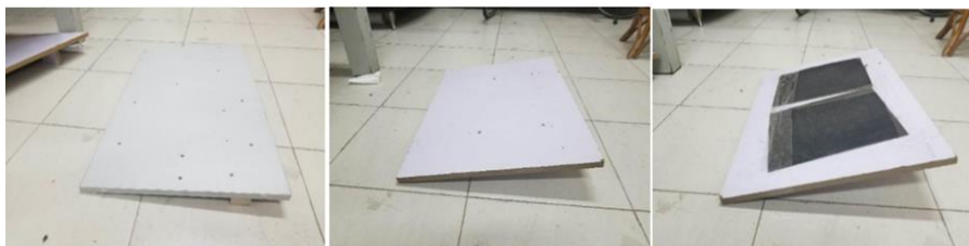
Fig. 1 5 °, 10 °, 15 ° inclined platform from left to right, the front of the toe is pointed to the right
