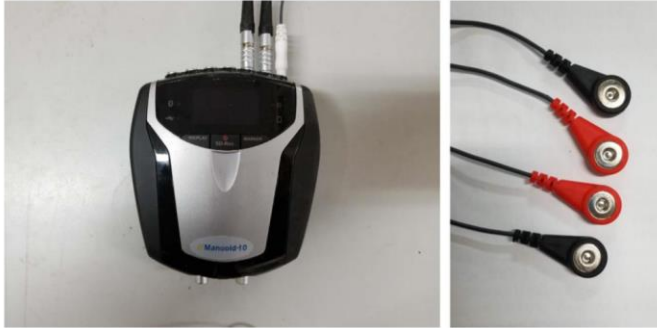
Fig. 2 Mangold-10 wireless Bluetooth multi-channel physiology system made in Germany
