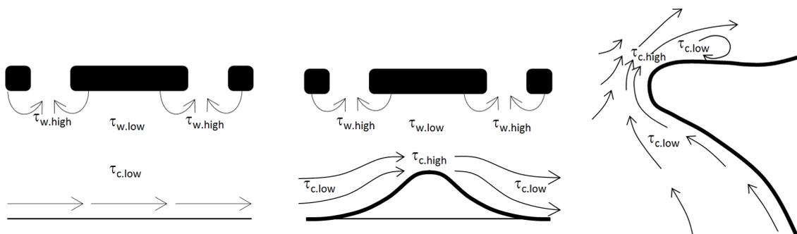
Figure 6. Conceptual feature development. (a) Dominant processes that result in the development of a cusped foreland (b) Change in bed shear stresses due to the development of the cusped foreland (c) Development of Point Maud by accelerated flow and a depositional eddy.
