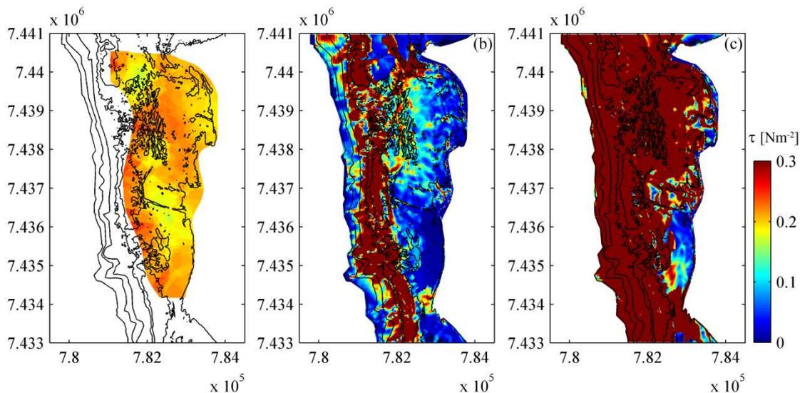
Figure 5. (a) The critical bed shear stress required to mobilize sediment based on the sediment grain size distributions. (b) The magnitude of the bed shear stress estimated by XBeach for moderate conditions ( $H_{rms} = 1$  m,  $T_p = 14$  s) (c) The magnitude of the bed shear stress estimated by XBeach for a storm condition ( $H_{rms} = 3$  m,  $T_p = 14$  s)
