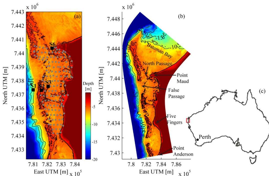
Figure 1. (a) Study site at Coral Bay with the locations of sediment grab samples (grey circles) and the location of hydrodynamic instruments (black squares). (b) Some key morphological features of Coral Bay. The depth of the bathymetry is indicated by the color bar. (c) Location of Coral Bay within Australia.
