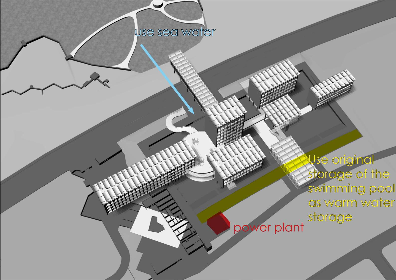
With a total of 4725 m2 the power plant is able to sustain 174 air conditioning at the same time. evaporate 1375L water/hour.
