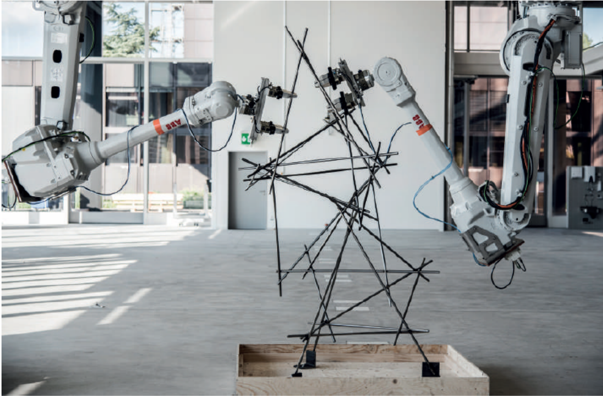
Figure 1.5: Example of an assembled structure by robotic arms [23]
