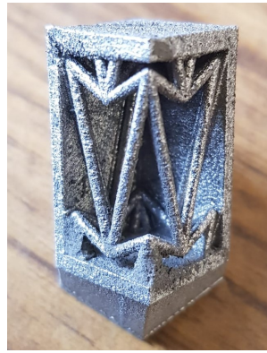
Figure 1.3: Double pyramid architecture created using SLM
