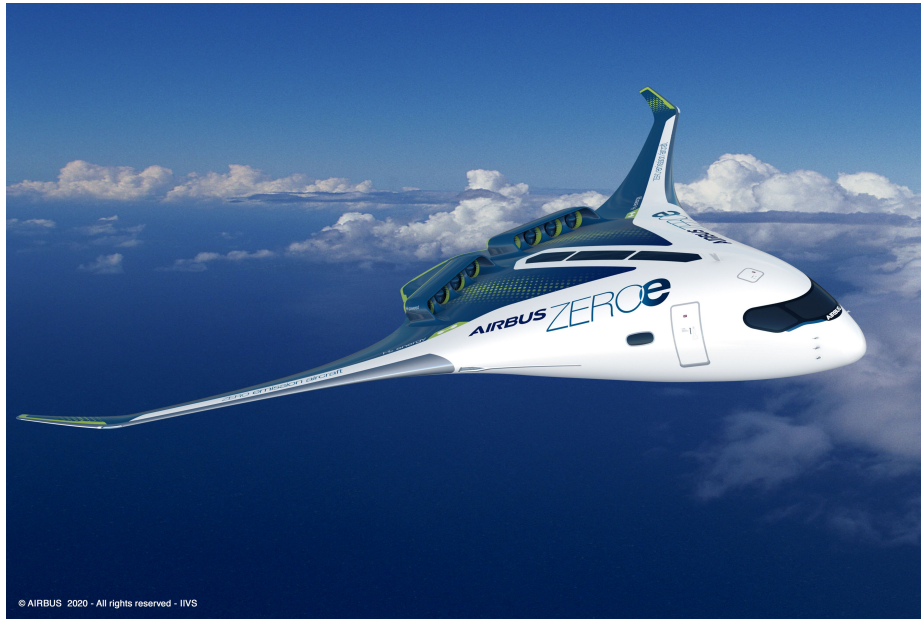
Figure 1.2: Airbus ZEROe small BWB concept announced in September 2020[4].
