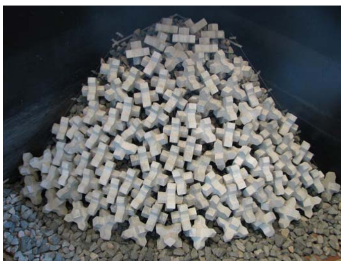
Figure 4.20 Packing Density Visual Inspection for Placement Test with Coherent Judgement
