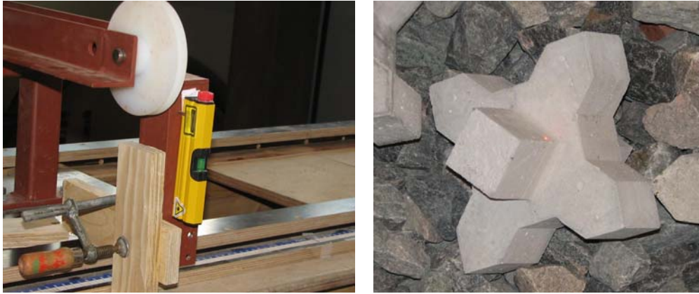
Figure 3.3 Laser Used for Measuring the Position of the Xbloc Unit
