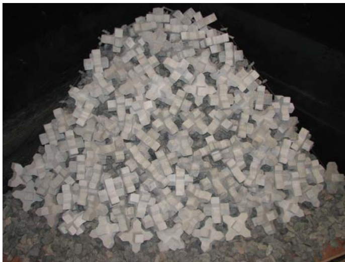
Figure 4.12 Packing Density Visual Inspection for recommended Design Grid Placement Tests
