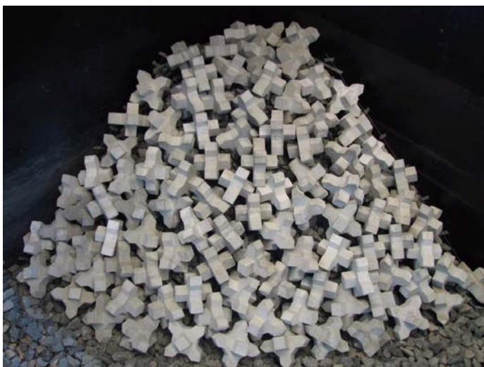
a) Test T1a Average Packing Density: 33.99 \text{ unit/m}^2 (93.84%) Standard Deviations: 7.8 \text{ unit/m}^2
