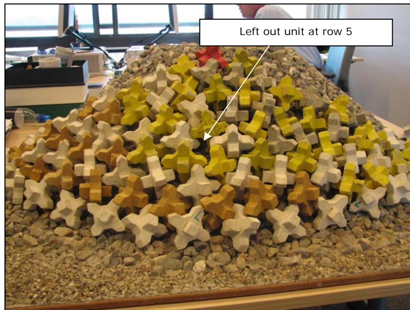
Figure 3.7 Starting point of the Left out Unit in Xbloc Trial Placement
