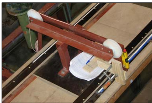
Top: Beam Platform on top of the basin. Right: Hoisting equipment to hold and position the unit.
