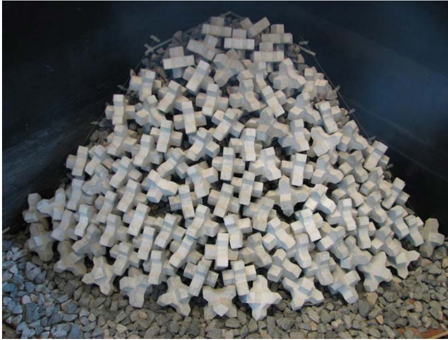
Figure 5.8 Xbloc Units Placements in TUDelft Laboratory: Test T2c
