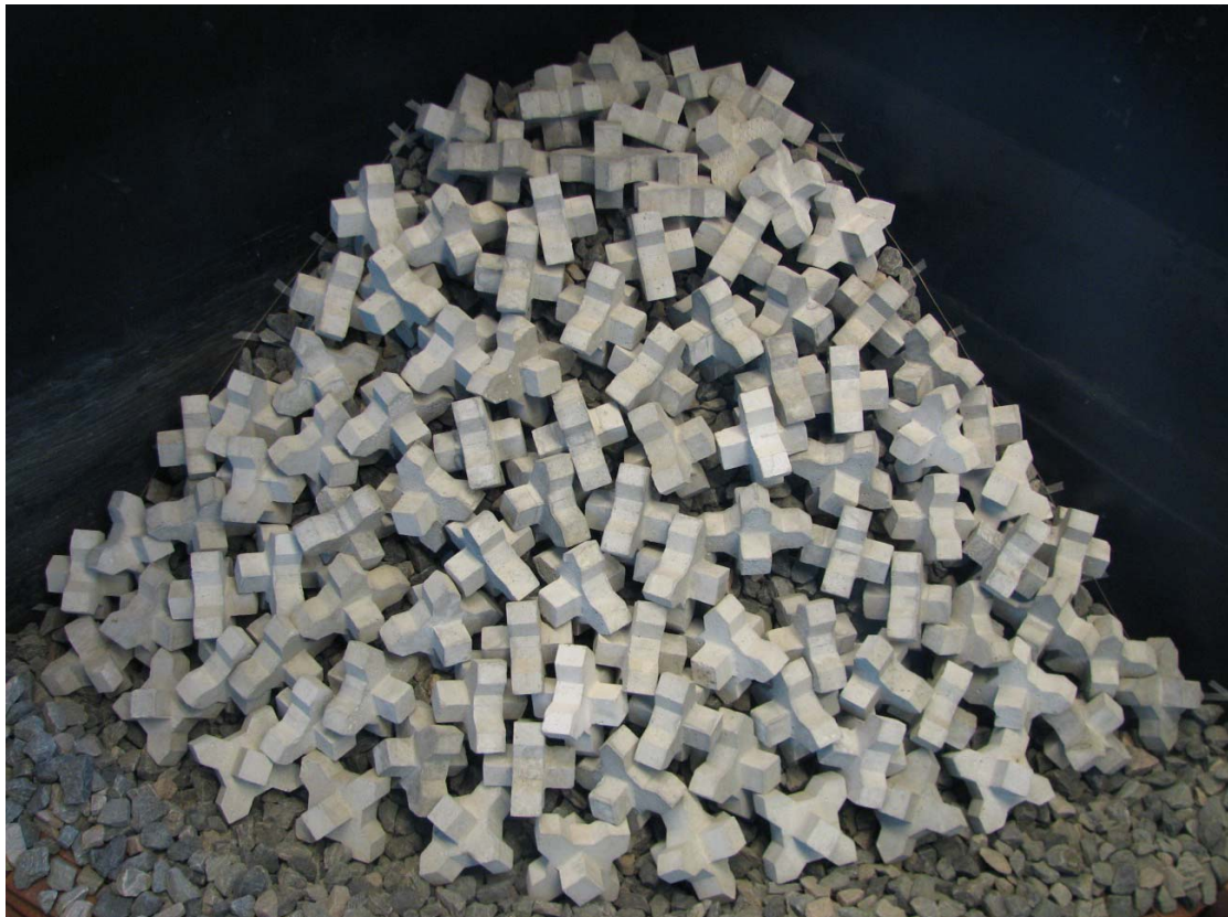
Figure 4.5 – Photograph of the Xbloc Recommended Placement Test T1b
