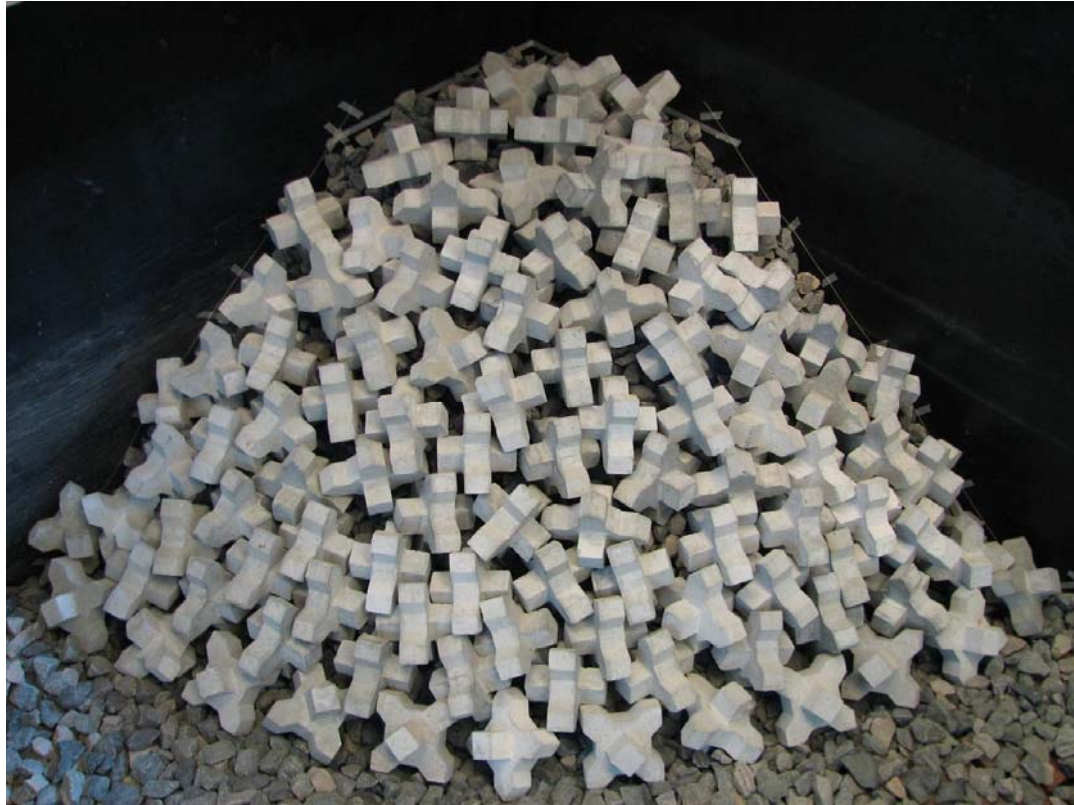
Figure 4.14 Photograph of the Xbloc Recommended Placement with Coherent Judgement Test T2b
