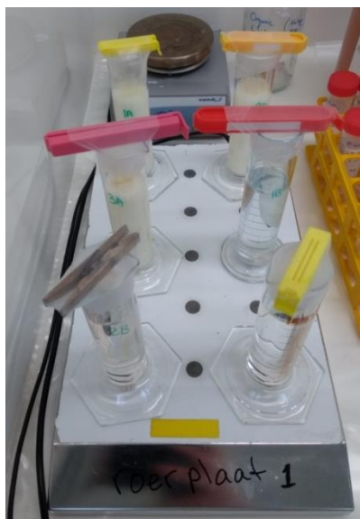
Figure 12: Setup for dialysis of milk. The graduated cylinders are placed on a stirring plate. The dialysis membrane is placed in the graduated cylinder. The clip makes sure that the dialysis membrane stays in place. The top of the graduated cylinder is covered with parafilm.
