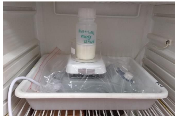
Figure 11: Setup to equilibrate milk, fortified with calcium carbonate ( \text{CaCO}_3 ), in the fridge.
