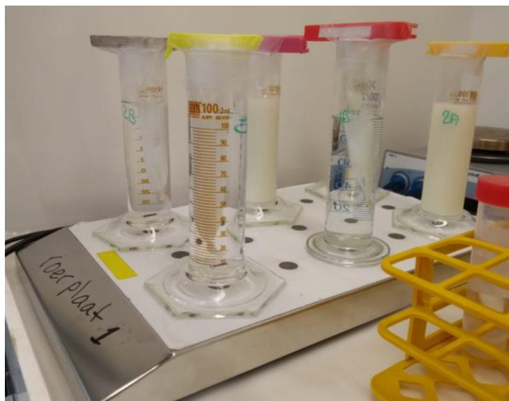
Figure 12: Setup for dialysis of milk. The graduated cylinders are placed on a stirring plate. The dialysis membrane is placed in the graduated cylinder. The clip makes sure that the dialysis membrane stays in place. The top of the graduated cylinder is covered with parafilm.
