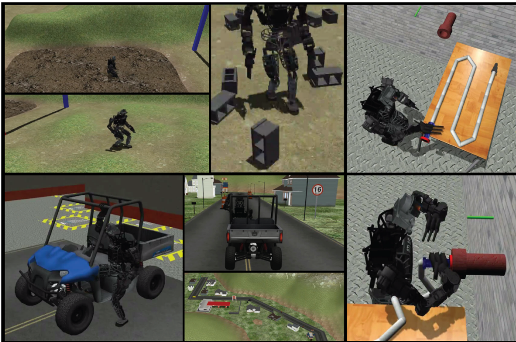
Figure 10. DARPA Virtual Robotics Challenge tasks. They included walking through mud, walking over hills, walking through debris, entering a vehicle, driving along a road, avoiding obstacles while driving, exiting a vehicle, picking up a hose, attaching the hose to a spigot, and turning on a valve.
