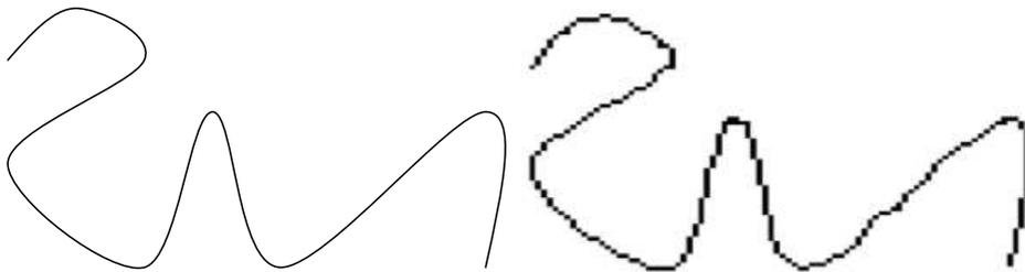
Fig. 3. Analogue representation of smoothly curved crack trace in a section (left) is replaced by an orthogonal set of straight line segments due to a conventional procedure of digitization (right).
