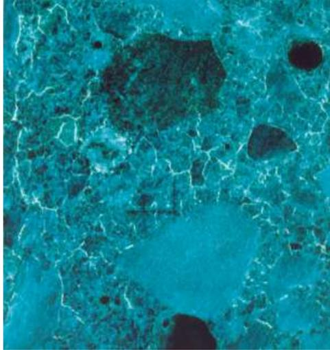
Fig. 4. Part of a cross-section of a pre-loaded concrete specimen reveals myriads of small cracks that are visualized by the fluorescent spray technique [8].
