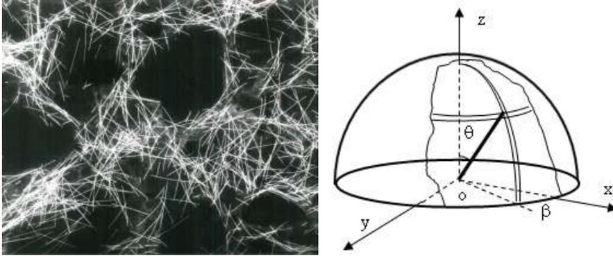
Fig. 7. Visualization by sphere model of orientation distribution of mono-size fibre elements (visualized for illustrative purposes in X-ray projection image (left)) in SFRC specimen. Fibre elements are considered translated from bulk to join in one of their ends in point O. As a consequence, other ends will UR cover the surface of the sphere with unit radius (right).
