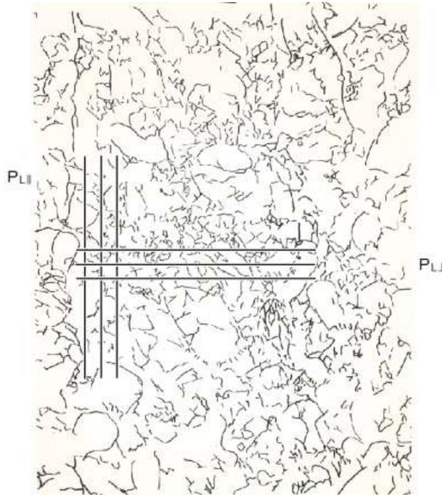
Fig. 5. Manually copied crack pattern of a full section image of a conventionally-sized prismatic concrete specimen (note the aggregate grain sections). Orthogonal line grids are superimposed for intersection direction counting, yielding measurements in horizontal and vertical directions, respectively (as indicated).
