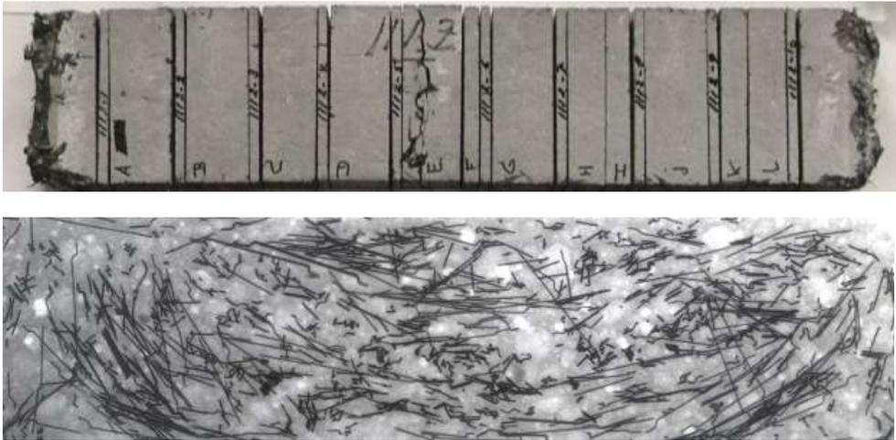
Fig. 6. SFRC specimen of 70x200x1000 mm (top) is sliced at regular distances to produce 10 tiles. An X-ray radiograph of such a “vertical slice” is shown at the bottom); gravitation during compaction was in vertical direction (perpendicular to top surface) [10].
