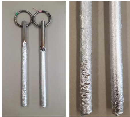
Figure 4-5: Pictures of the sample rods taken out the bath. Left rod is sample 1.3 (GI+MZ+GI), the right rod is sample 1.1 (GI only)
