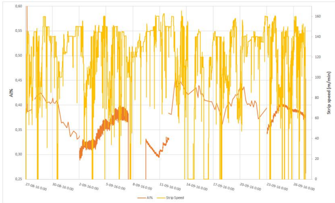
Figure 3-4: DVL3 process speed during the hardware campaign. The process stopped several times, which seems to have no effect on the Al%
