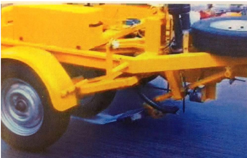
Figure 2.8 Measurement system for the skid resistance [Gaarkeuken, 2006]
