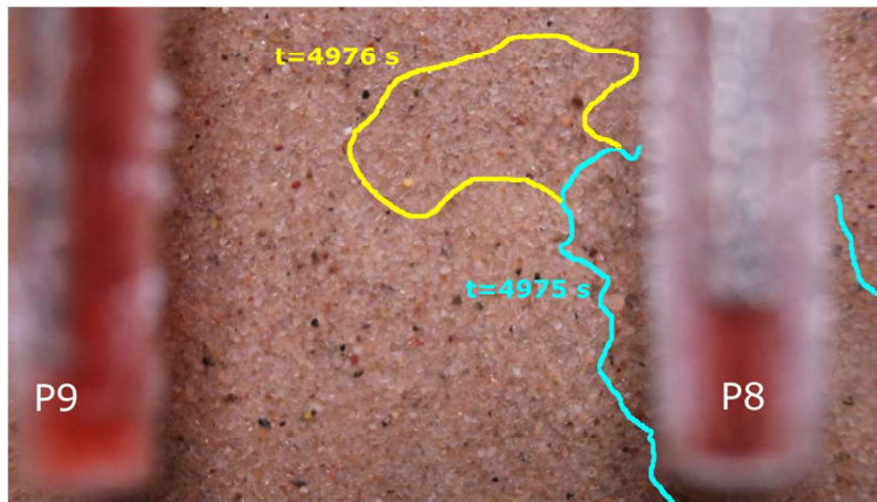
Figure 4. Zone around pipe tip in test B25_245 s just before (t=4975s) and during (t=4976s) second group detachment.
