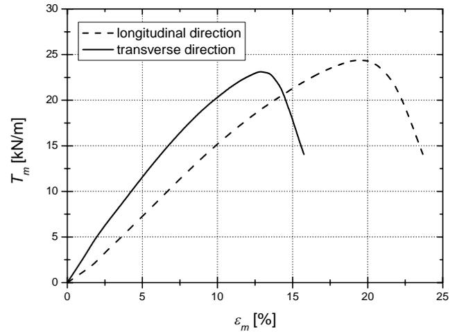
Figure 4. Tensile strength *versus* strain behaviour in longitudinal and transverse directions of the model synthetic.
