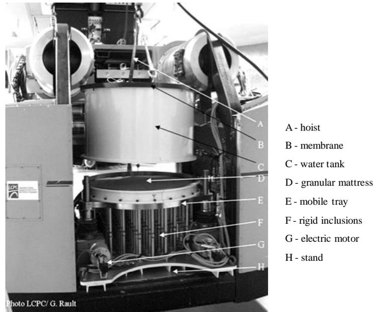
Figure 6. General view of the mobile tray device inside the basket of the centrifuge.
