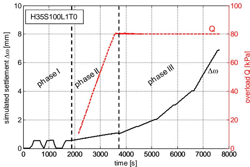
Figure 7. Mobile tray displacement  $\Delta\omega$  under its center and overload  $Q$  applied to the granular mattress during the three phases of the test H35S100L1T0.
