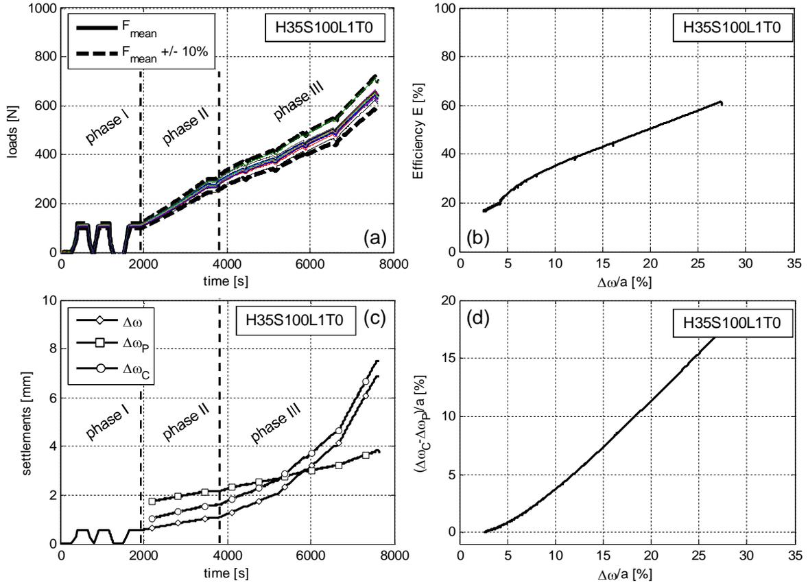
Figure 8. Evolutions of (a) loads  $F$  in the nine instrumented piles with the time - (b) the efficiency of the load transfer mechanism as a function of the ratio  $\Delta\omega/a$  - (c) the settlements of the soft soil simulated by the tray  $\Delta\omega$ , above the central pile  $\Delta\omega_P$  and the centre of an unit cell  $\Delta\omega_C$  with the times - (d) the dimensionless differential settlement as a function of the ratio  $\Delta\omega/a$  (test H35S100L1T0).
