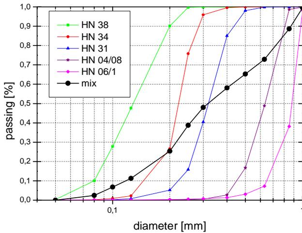
Figure 3. Grading curve of the model granular mattress made from five fractions of Hostun sand (HN38, HN34, HN31, HN04/08 and HN06/1).
