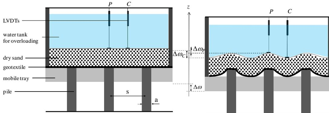
Figure 9. Schematic view of settlements measurements: above the central pile (point  $P$ ,  $\Delta\omega_P$ ) and at the middle of an unit cell (point  $C$ ,  $\Delta\omega_C$ ) - before (left) and during (right) the mobile tray down  $\Delta\omega$ .
