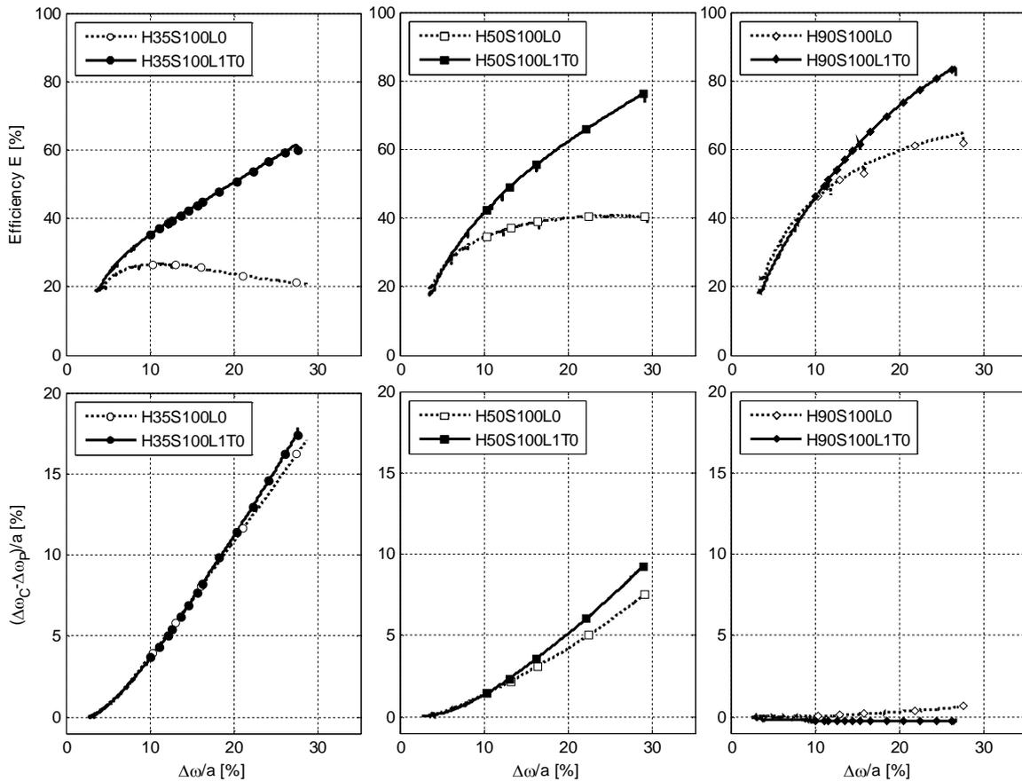
Figure 11. Comparison with and without geosynthetic reinforcement of the efficiency  $E$  and of the dimensionless differential settlement  $(\Delta\omega_C - \Delta\omega_P)/a$  for the three granular mattress thickness:  $H = 35$  mm (left) -  $H = 50$  mm (middle) and  $H = 90$  mm (right).
