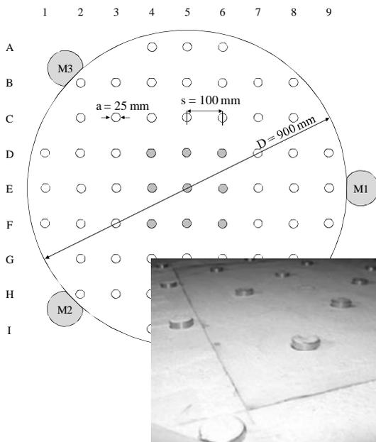
Figure 5. Schematic representation of the mobile tray and a close picture showing glued rough sandy interface.
