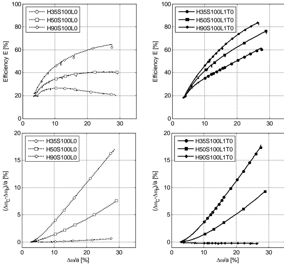
Figure 10. Evolutions of the efficiency  $E$  and of the dimensionless differential settlement  $(\Delta\omega_c - \Delta\omega_p)/a$  versus  $\Delta\omega/a$  for the three reference tests “LO” (left) and the three tests with a geosynthetic layer “L1T0” (right) for  $H = 35, 50$  and  $90$  mm.
