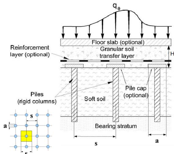
Figure 1. Components of the pile supported earth platform system (Simon and Schlosser, 2006) and definition of a unit cell in a pile mesh.
