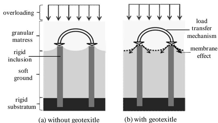
Figure 2. Schematic representations of the load transfer mechanisms in a granular - (a) without geotextile - (b) with a geotextile layer.
