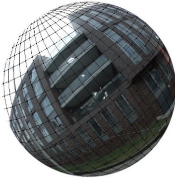
Figure 2. A panoramic image on a sphere. The lines represent latitude and longitude.
