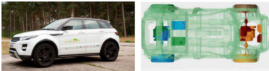
Fig. 1. SUV demonstrator with individual on-board motors.
