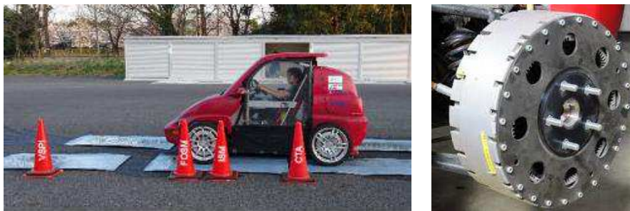
Fig. 5. Vehicle demonstrator FPEV2-Kanon with four individual in-wheel motors.
