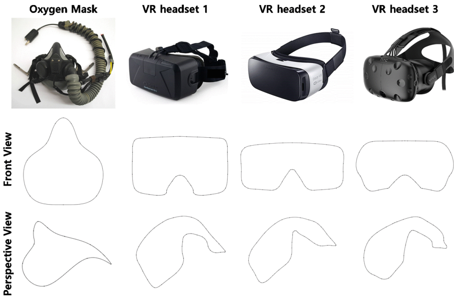
Fig. 4. Facial wearable products and its spline curvature in front and perspective views.
