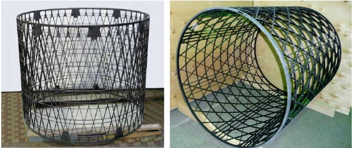
Figure 3-5 Lattice cylinders with irregular helical rib pattern, produced by wet filament winding [1]
