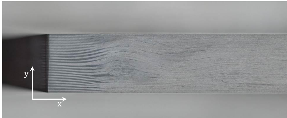
Figure 5-30 Micro-section of a helical rib joining a hoop rib, showing typical ply waviness
