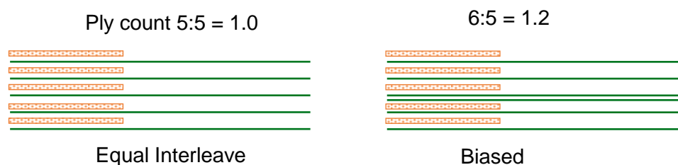
Figure 6-7 Schematic showing different interleave ratios
