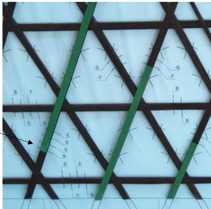
Figure 5-12 Rib width transitions using a gradual build up, where ply drops occur at the mid rib
