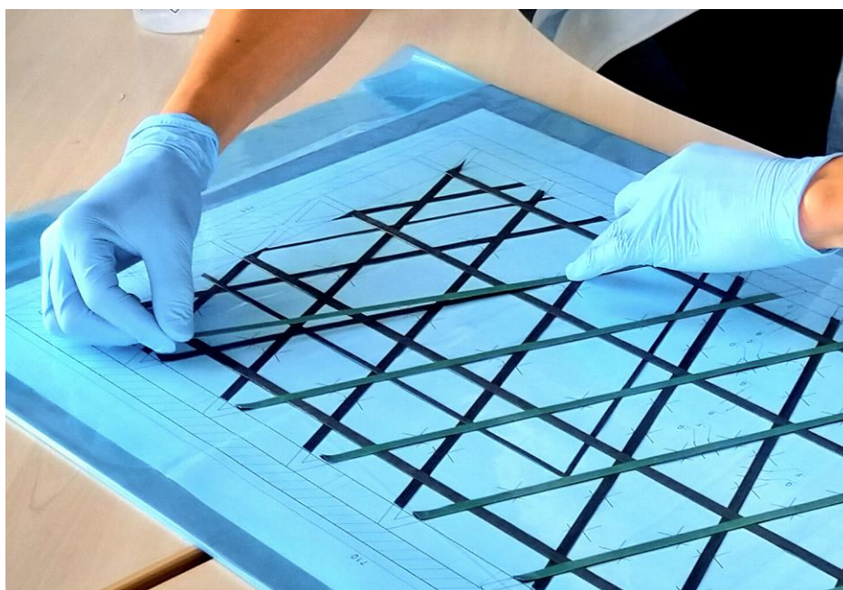
Figure 5-3 Manual tow layup showing light consolidation at tow intersections and layup template
