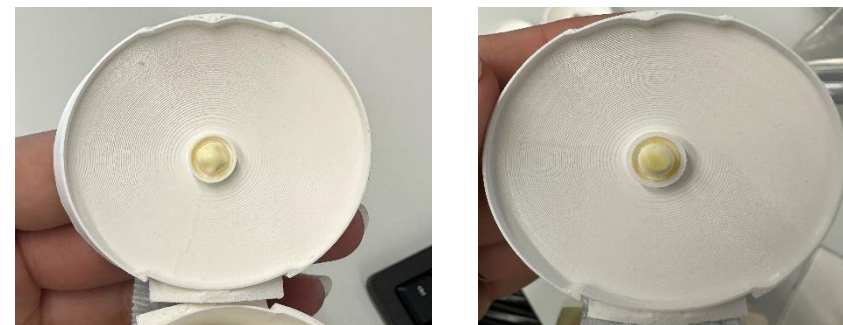
Figure 80. Cleanness of the previous pin design (L) and new design (R).
