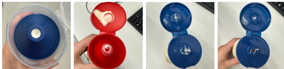
Figure 34. Cleanness inside the closure after squeezing (L-R, MPS=1, Interkap=5, Latam =4, 4 mm orifice = 3.)
