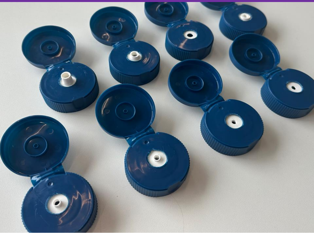
Figure 56. tested prototype insert in the Latam closure (Heinz, AH and shampoo)
