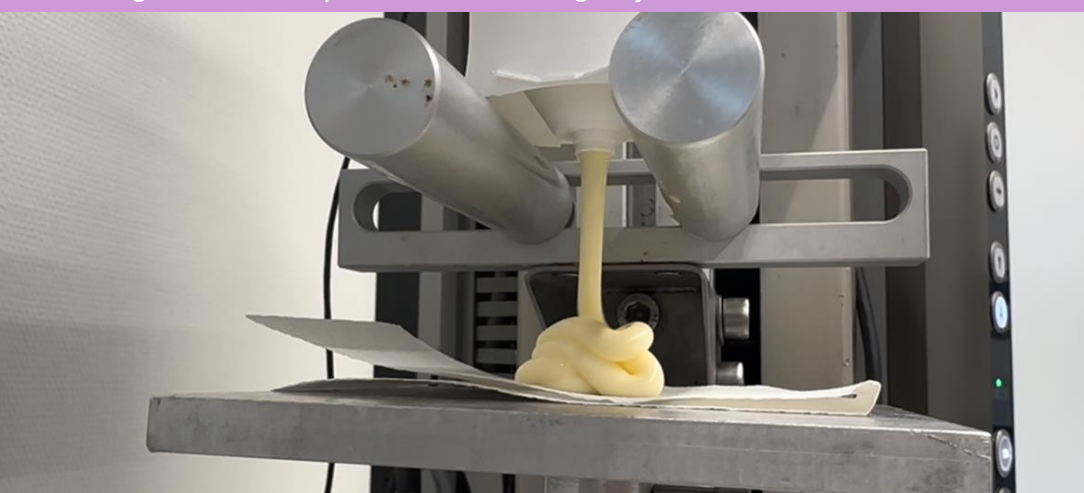
Figure 77. Squeeze test of a MPS bottle with the designed and 3D-printed closure Figure 78. The 3D-printed closure dosing mayonnaise
