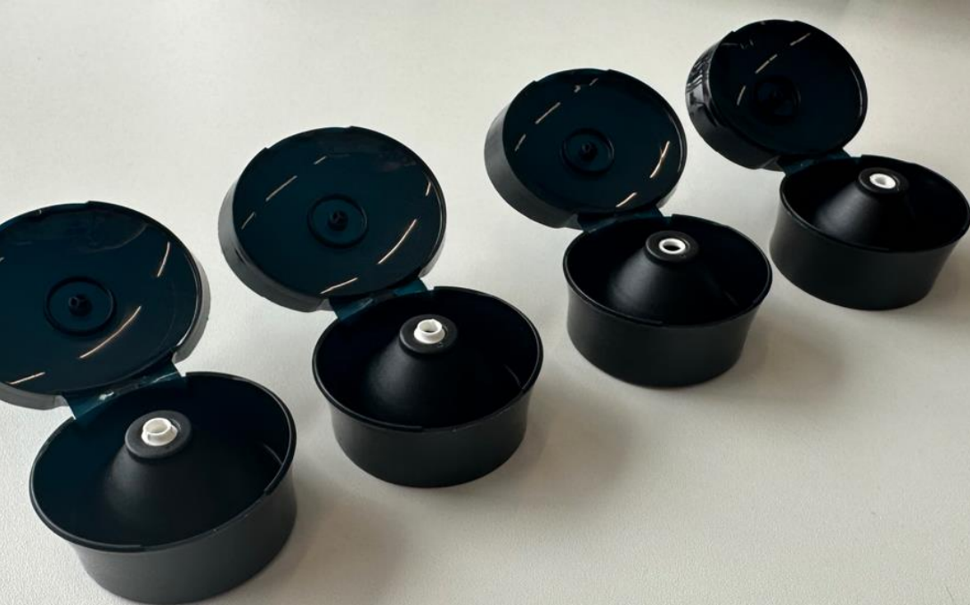
Figure 55. tested prototype inserts in the MPS closure (Heinz designs)
