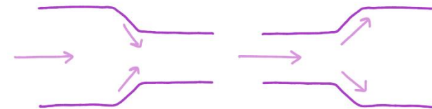
Figure 66. Flow from a large area to a small area (L), flow from a small area to a large area (R).
