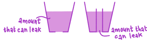
Figure 71. Inside tube will decrease the chance of leaking.
