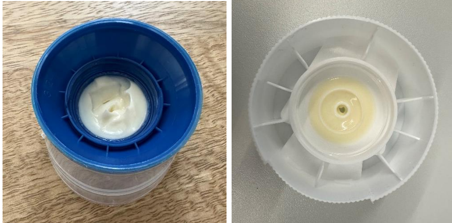
Figure 42. looks inside the closure after squeezing (MPS Left – Heinz Right)
