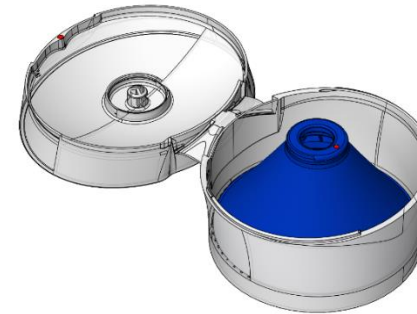
Figure 106. Overview of the two injection points on the original MPS closure.
