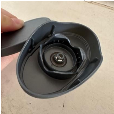
Figure 18. Bridge with hole orifice.
