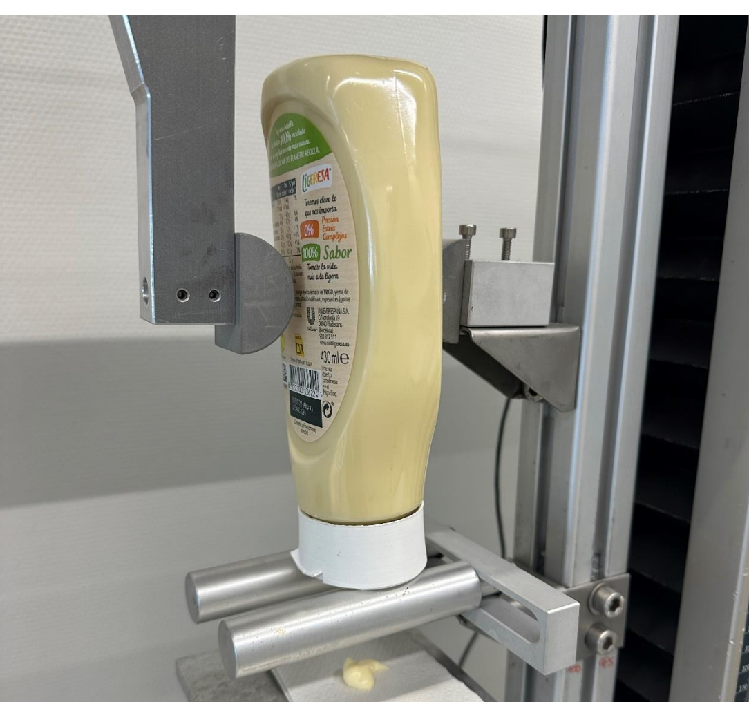
Figure 77. Squeeze test of a MPS bottle with the designed and 3D-printed closure Figure 78. The 3D-printed closure dosing mayonnaise
