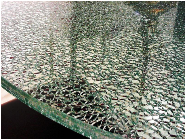
Post-breaking structural capacity of panel
