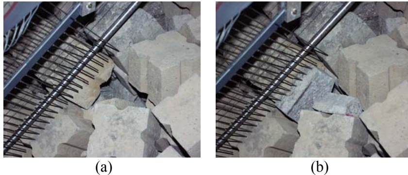
Figure 14: Hole between cubes: (a) original pattern, (b) hole partly filled.
