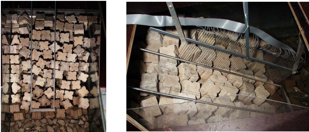
Figure 11: Run-up gauges: (a) sloping gauges, (b) step gauge.
